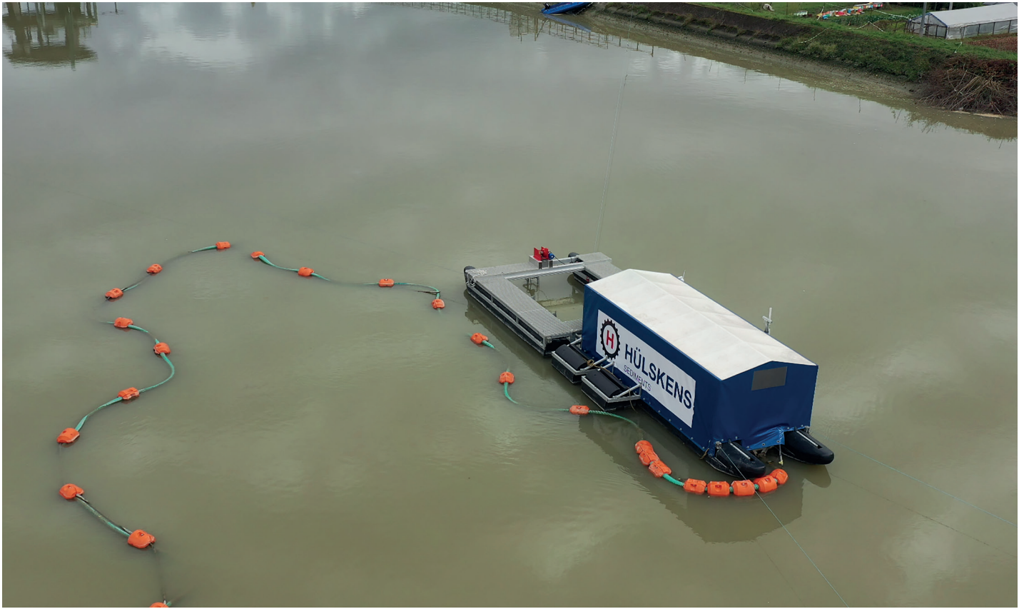
FIGURE 4 SediMover-130 at a project in Italy during continuous sediment transfer.
