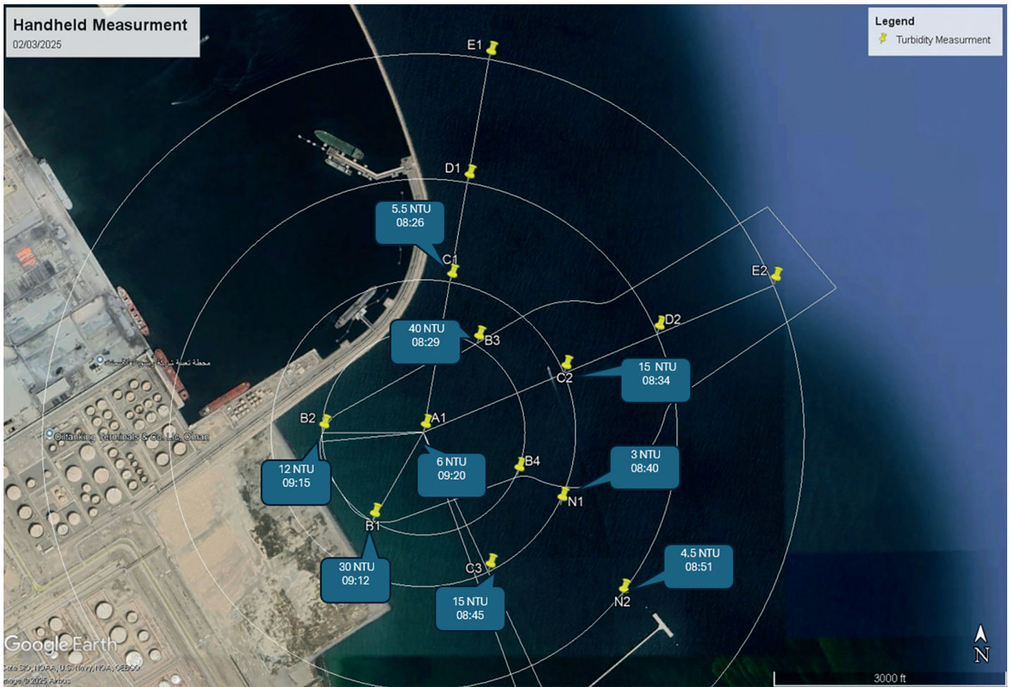
FIGURE 7 Example of handheld measurements during project execution.
