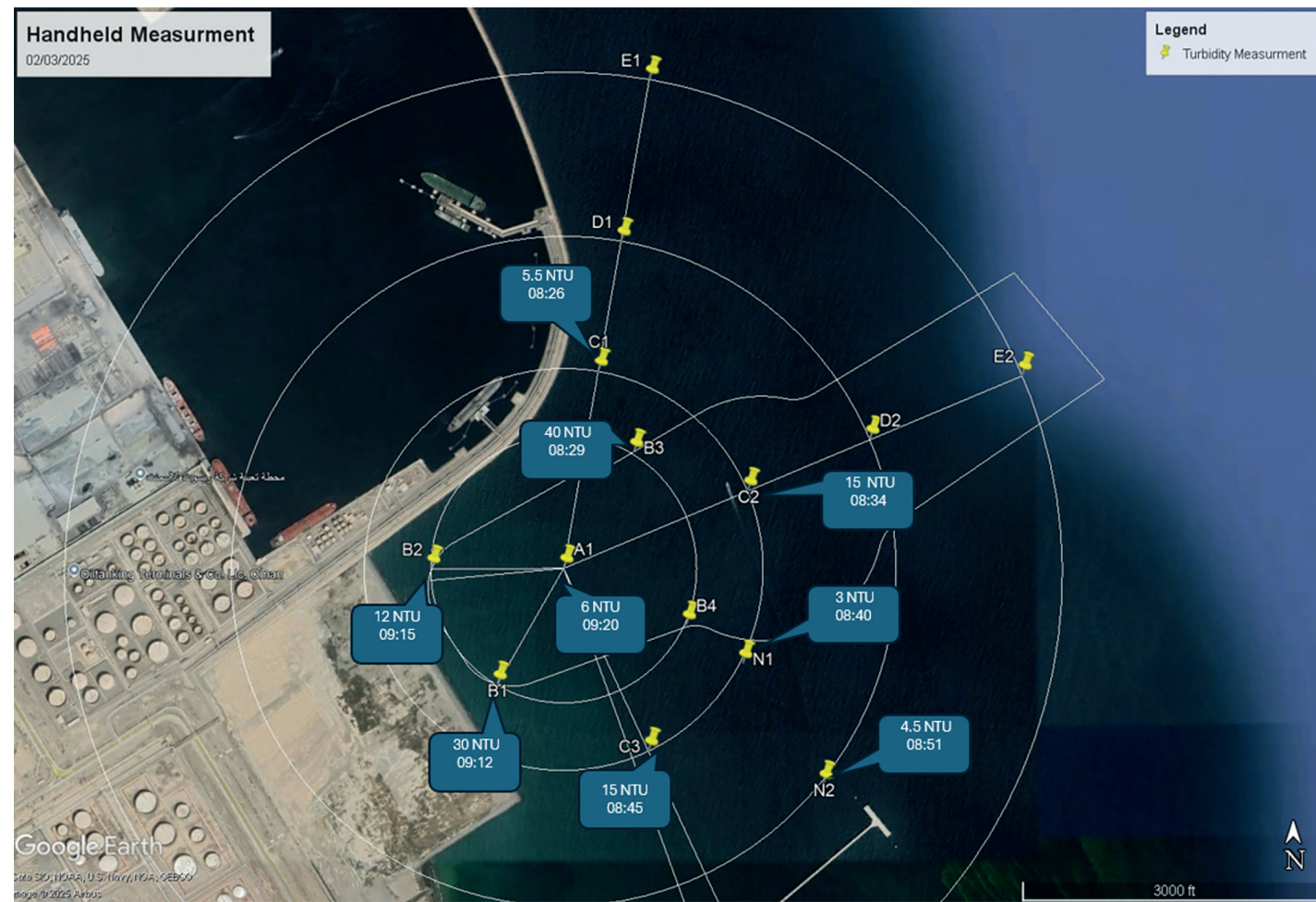
FIGURE 7 Example of handheld measurements during project execution.
