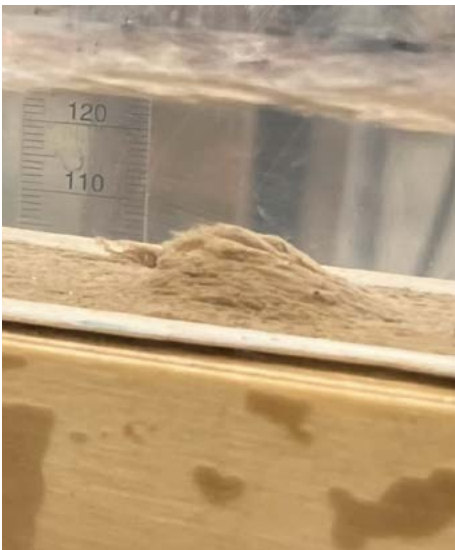
FIGURE 4 Local accumulation during the longitudinal flow tests.
