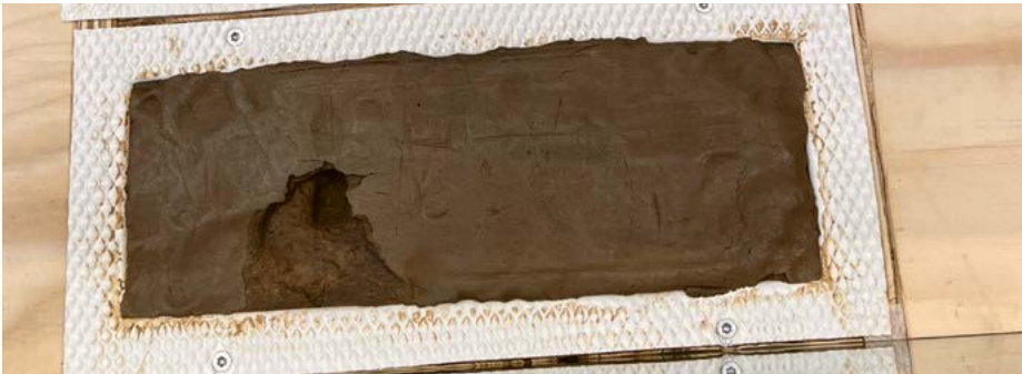
FIGURE 13 Clay CAT. 1 sample during test 1.
