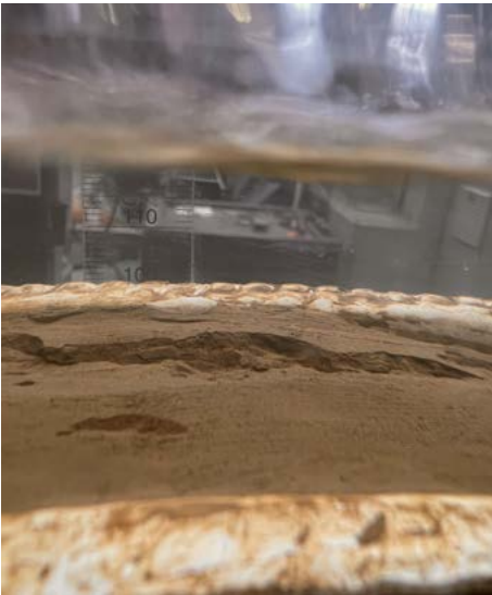
FIGURE 7 Erosion clay CAT. 1 during longitudinal flow tests.
