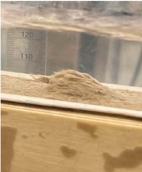
FIGURE 4 Local accumulation during the longitudinal flow tests.
