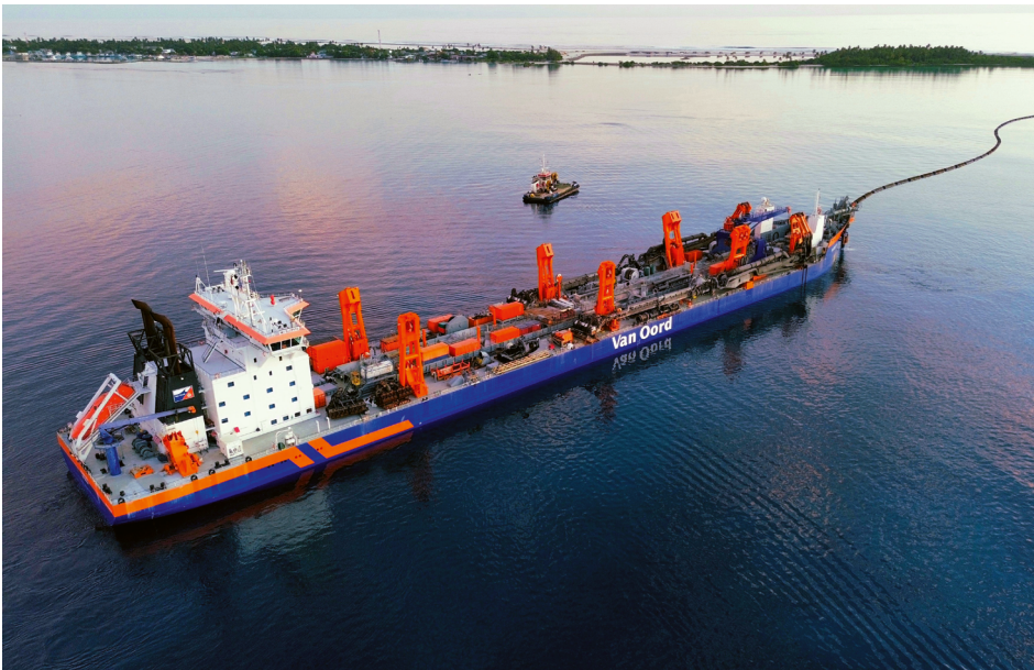
FIGURE 4 The trailing suction hopper dredger HAM 318 in Addu City, Maldives during reclamation of Hithadhoo zone 2.
