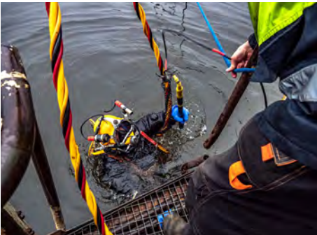
FIGURE 13 UXO trained diver using handheld magnetometer.
