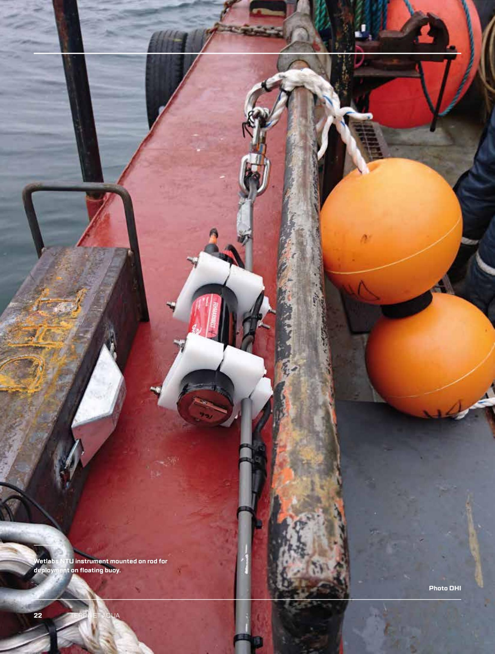
Wetlabs NTU instrument mounted on rod for deployment on floating buoy.
