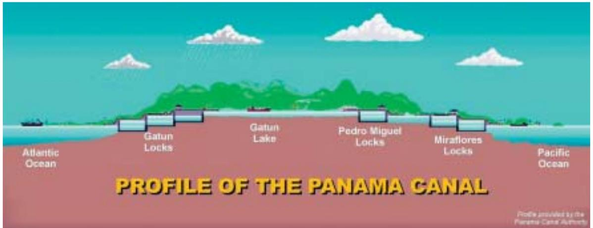
Figure 3. Profile of the Panama Canal, showing the locks and lakes that connect the two oceans.
