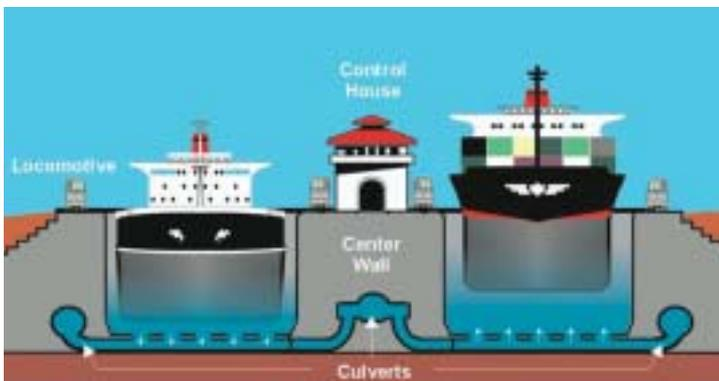
Figure 4. A cross-section of the Canal locks.
