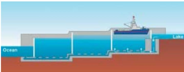
Figure 5. Elevation of the Canal locks chambers.
