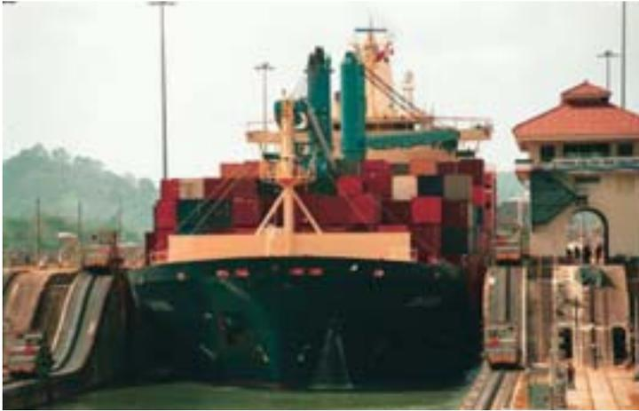
Figure 8. A Panamax vessel going through a lock with very little room to spare.
