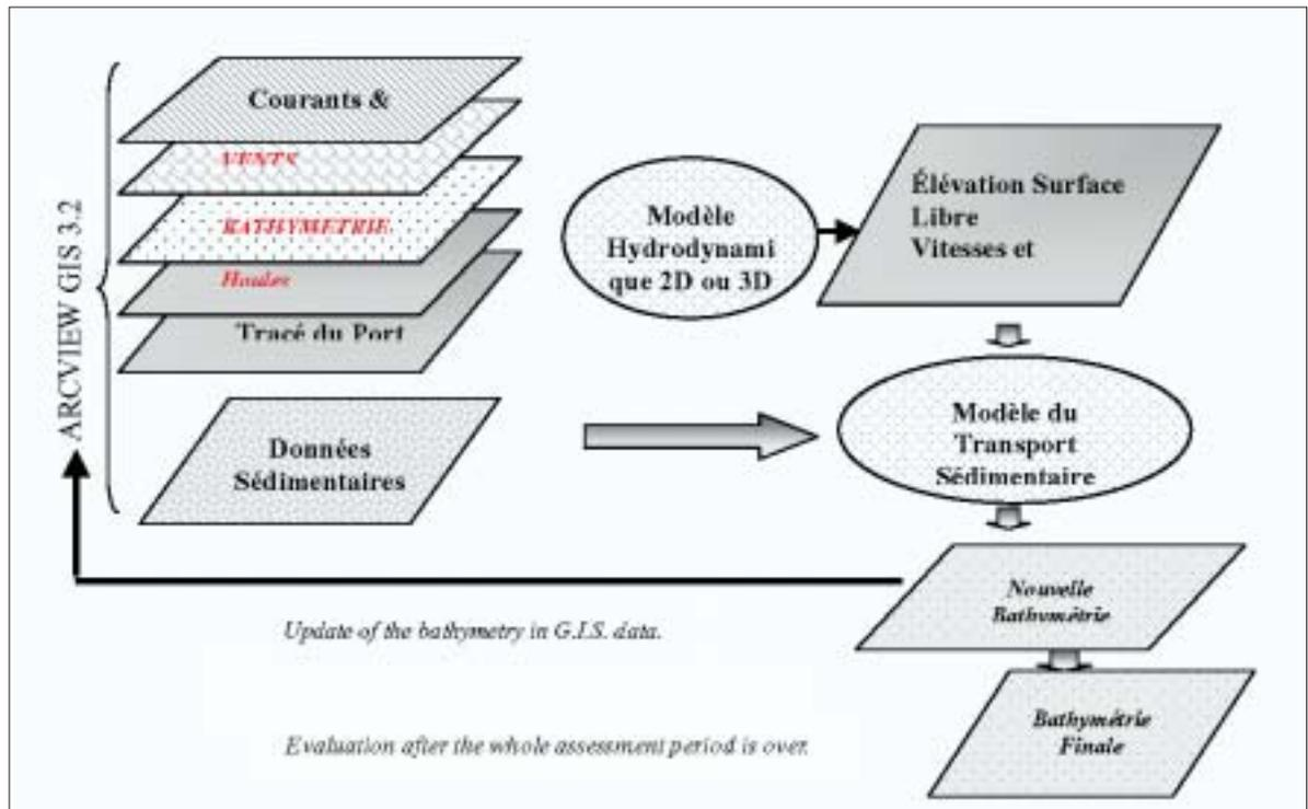
Figure 6. Design scheme of the prediction model of sand encroachments and erosions.
