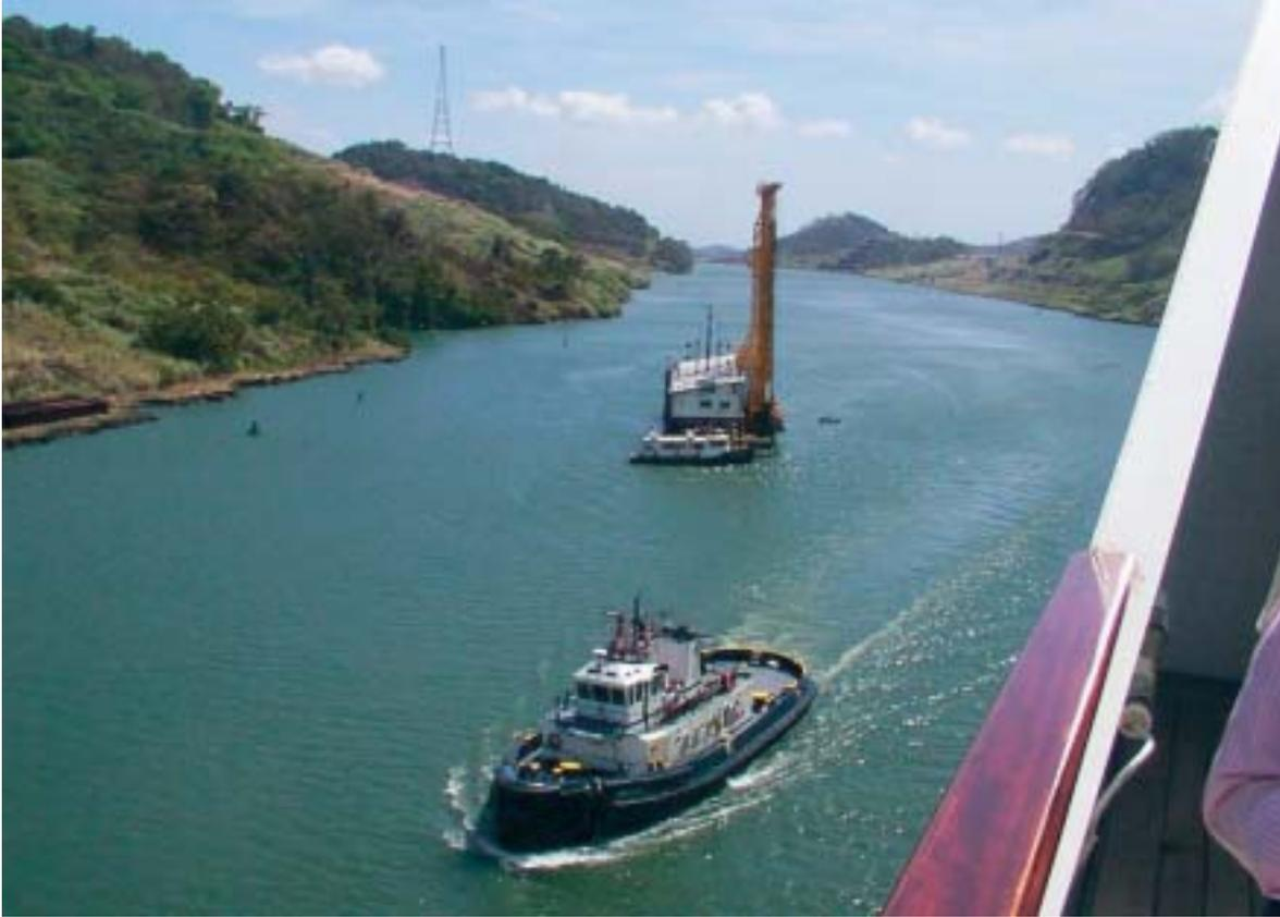
Figure 13. Drillboat Thor working in the Gaillard Cut on the next phase of deepening the cut to increase water storage in Gatun Lake. Six-inch holes are drilled, filled with dynamite and blasted. The fractured rock is then removed by the dipper dredger Rialto M. Christensen.
