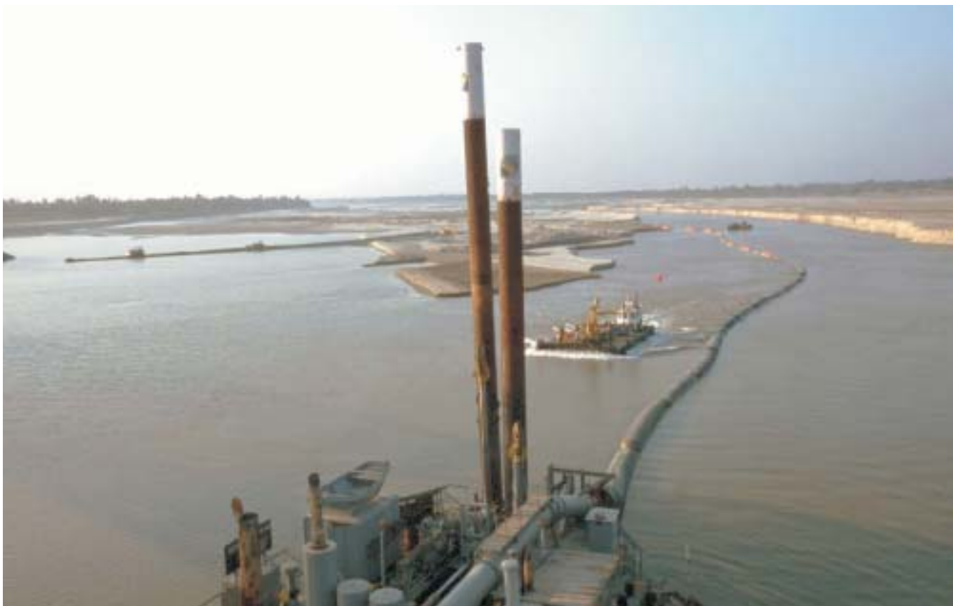
Figure 4. Aerial view of the cutter suction dredger at work.
