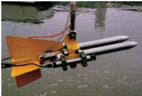
Figure 3. Picture of towfish (Navitracker equipped with OBS sensors).
