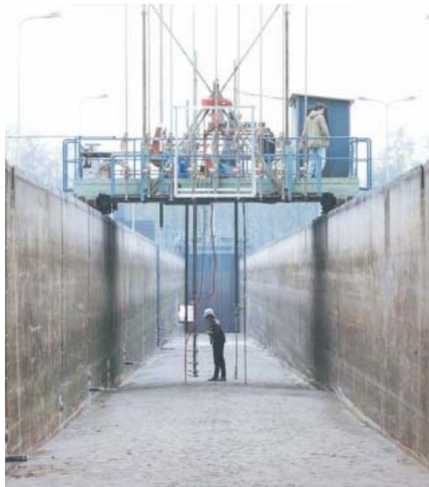
Figure 7. Measurement carriage used during the LIP 11D programme in the Delta flume.
