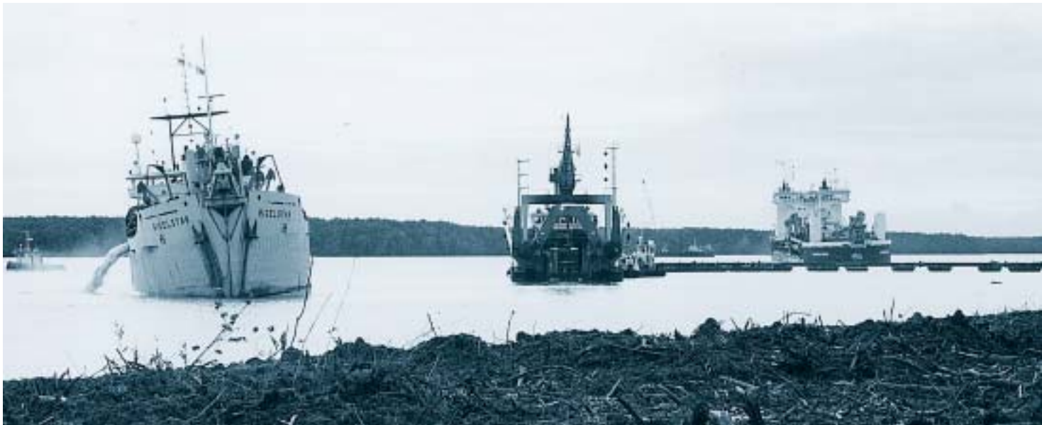
Figure 6. A large fleet of dredging vessels were used simultaneously: Seen here, trailing suction hoppers Rigelstar (left) and Amsterdam (right) were joined by cutter dredgers such as the Hector (center).
