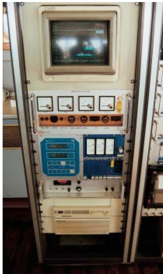
Figure 11. Monitoring system on board a dredger is a necessary part of the auditing system which forms the basis for the environmental review.
