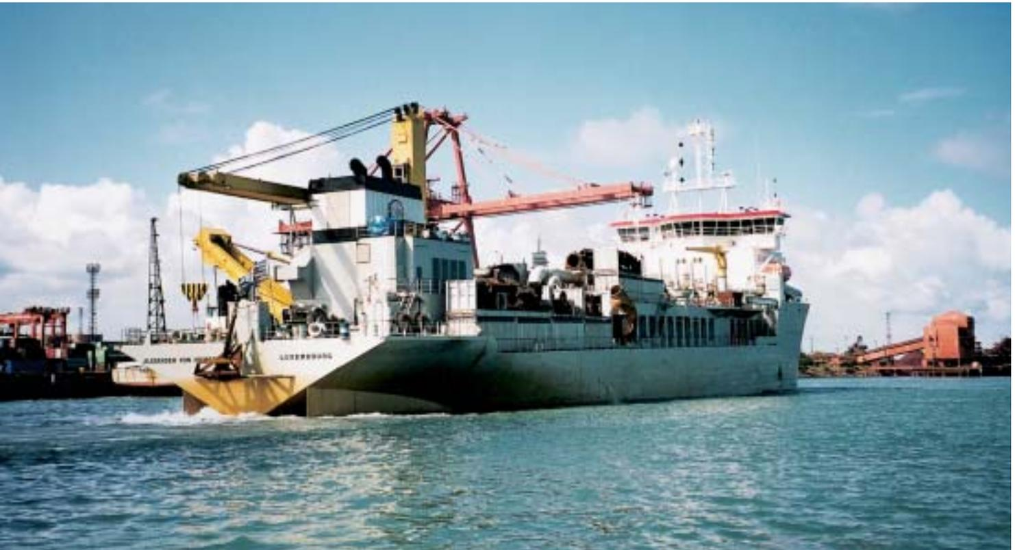
Figure 5. The 9,000 m<sup>3</sup> trailing suction hopper dredger *Alexander von Humboldt*, has been commissioned to the Ennore Port Project for dredging the 3,525-m-long Access Channel.
