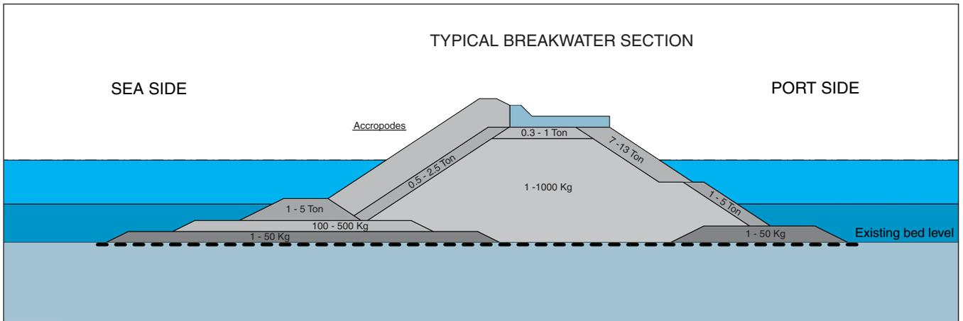
Figure 1. A cross-section of a typical breakwater.
