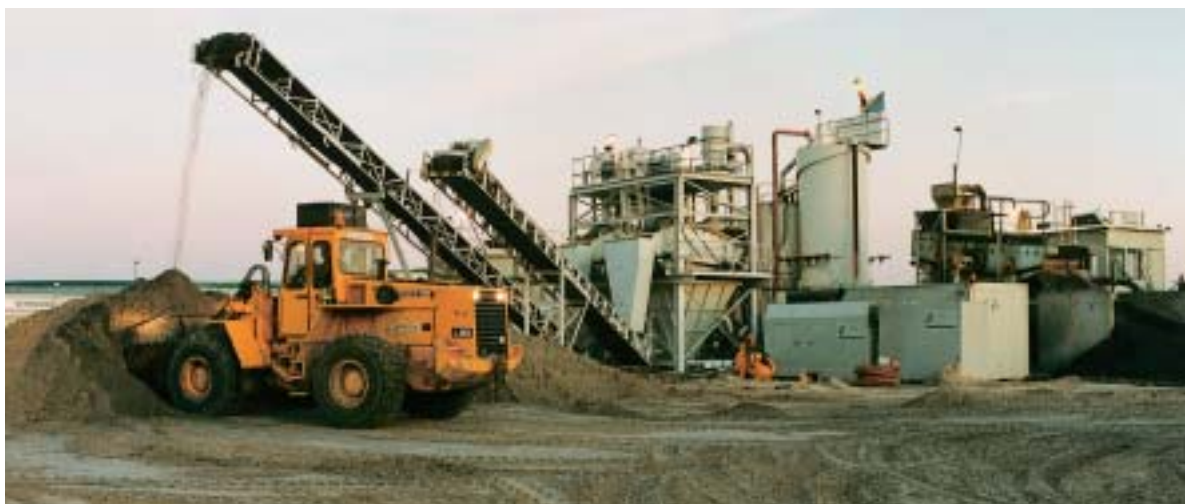
Figure 2. At this dry sediment treatment plant in Rotterdam's Maasvlakte, contaminated sediment is washed and de-watered. The processed clean sand can be reused for construction projects.
