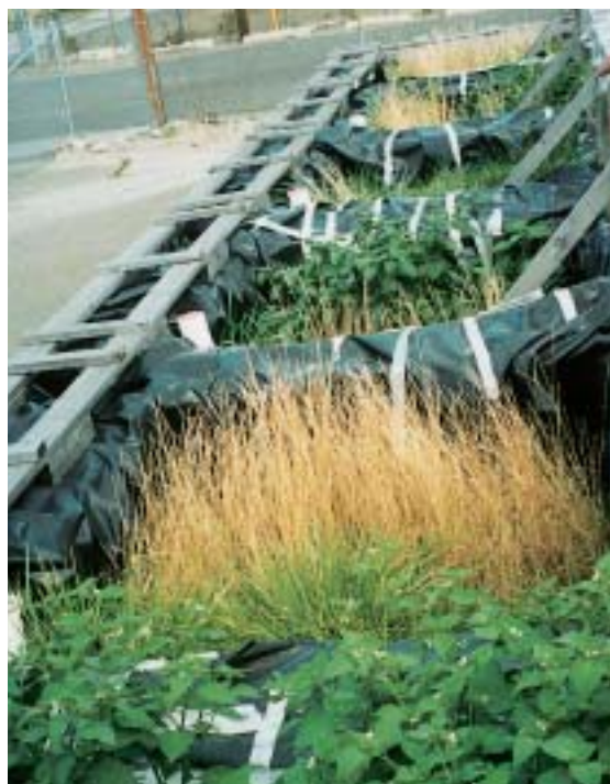
Figure 3. An experiment in growing vegetation on treated dredged material in the USA.
