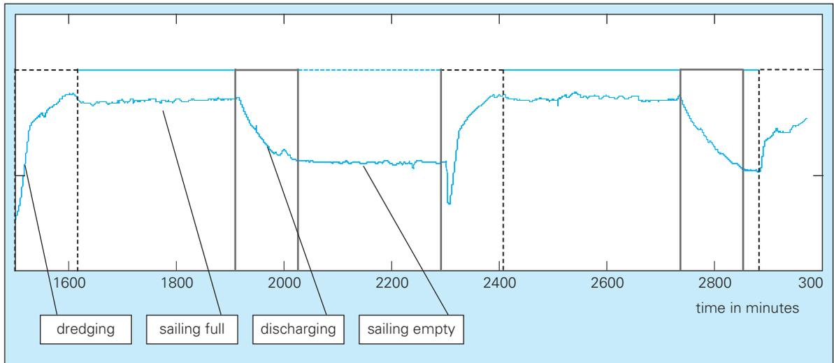
Figure 2. Displacement and status signals versus operational time.
