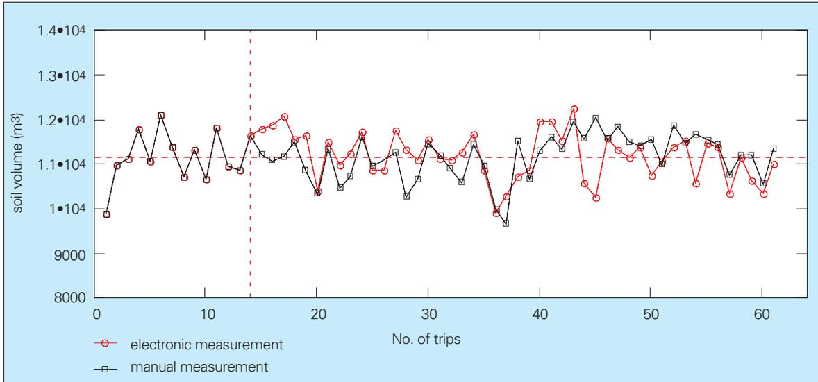
Figure 3. Volume measurement, hopper dredger Amsterdam.
