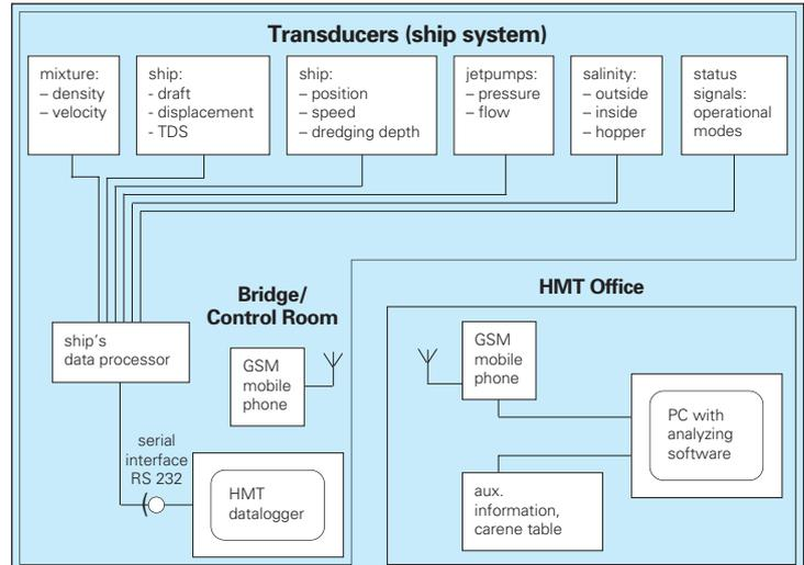
Figure 1. Basic sketch of hopper operation monitoring with remote data acquisition system.
