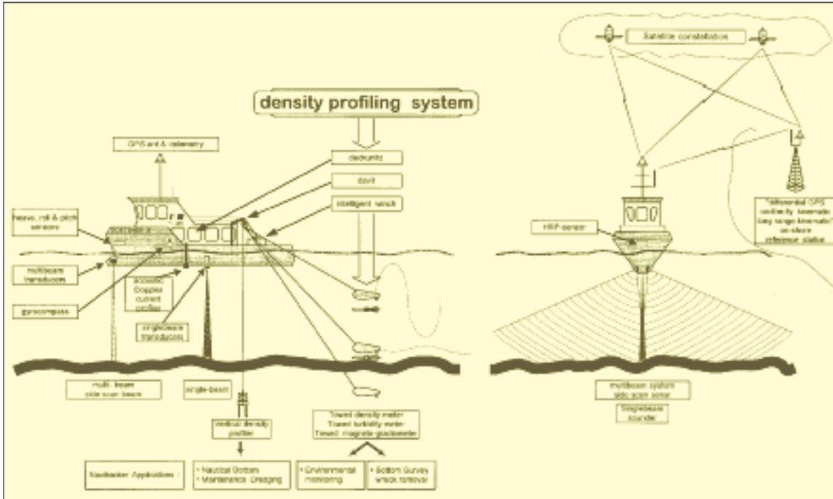
Figure 1. Survey vessels and systems: general application programme.
