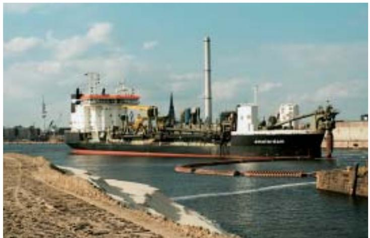
Figure 4. The Amsterdam working on harbour filling in Hamburg.
