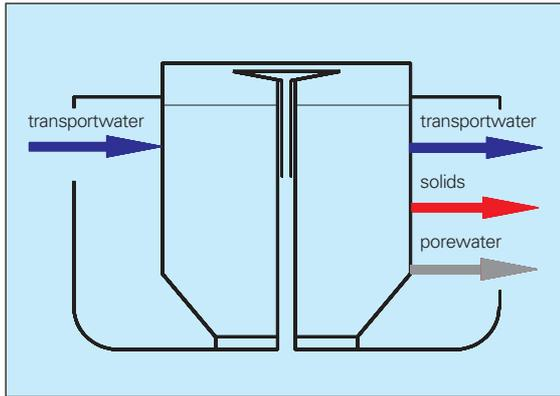
Figure 5. Mass balance during hopper discharge.
