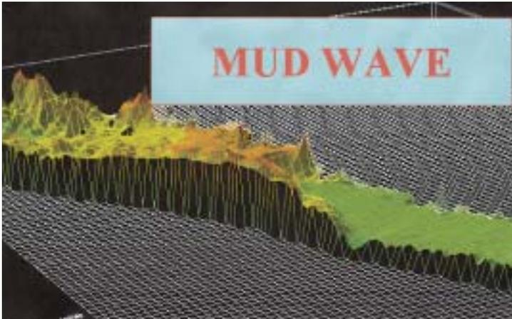
Figure 3. In fluid mud areas, deep-draughted vessels sail above a clearly defined physical (density) level within the fluid mud body. Although an internal wave is observed at the sediment-water interface, safe navigation is not hampered and is guaranteed by the navigable depth concept.
