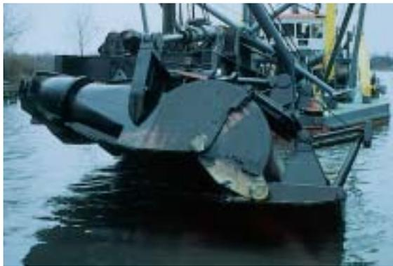
Figure 3. The dredger Vlaanderen XV equipped with the sweephead.
