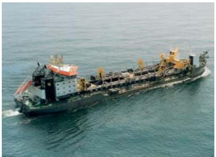
Figure 6. In June 1997 the WD Fairway became the world's largest trailer with a hopper capacity of 23,425 m<sup>3</sup>.
