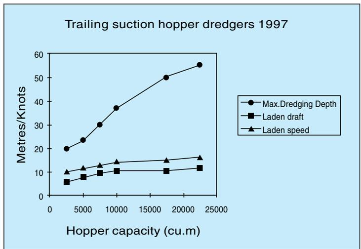
Figure 10. Characteristics of trailing suction hopper dredgers in 1997.
