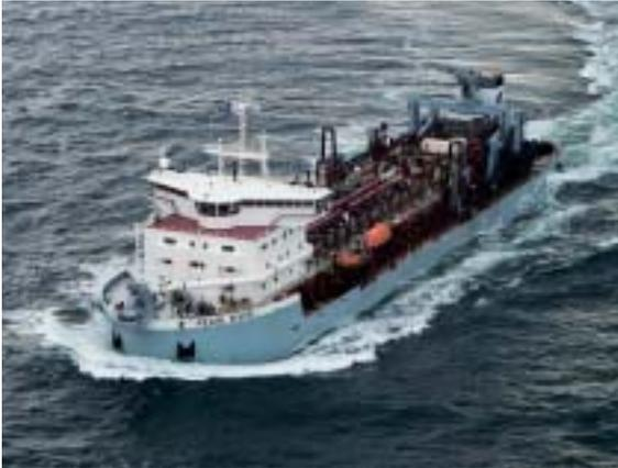
Figure 3. The Pearl River (17,000 m<sup>3</sup>), built in 1994, is one of the largest TSHDs in the world.
