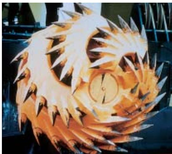
Figure 2. View of a traditional cutter crown.
