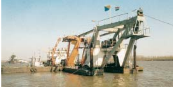
Figure 1. Suction dredger Groningen at work.
