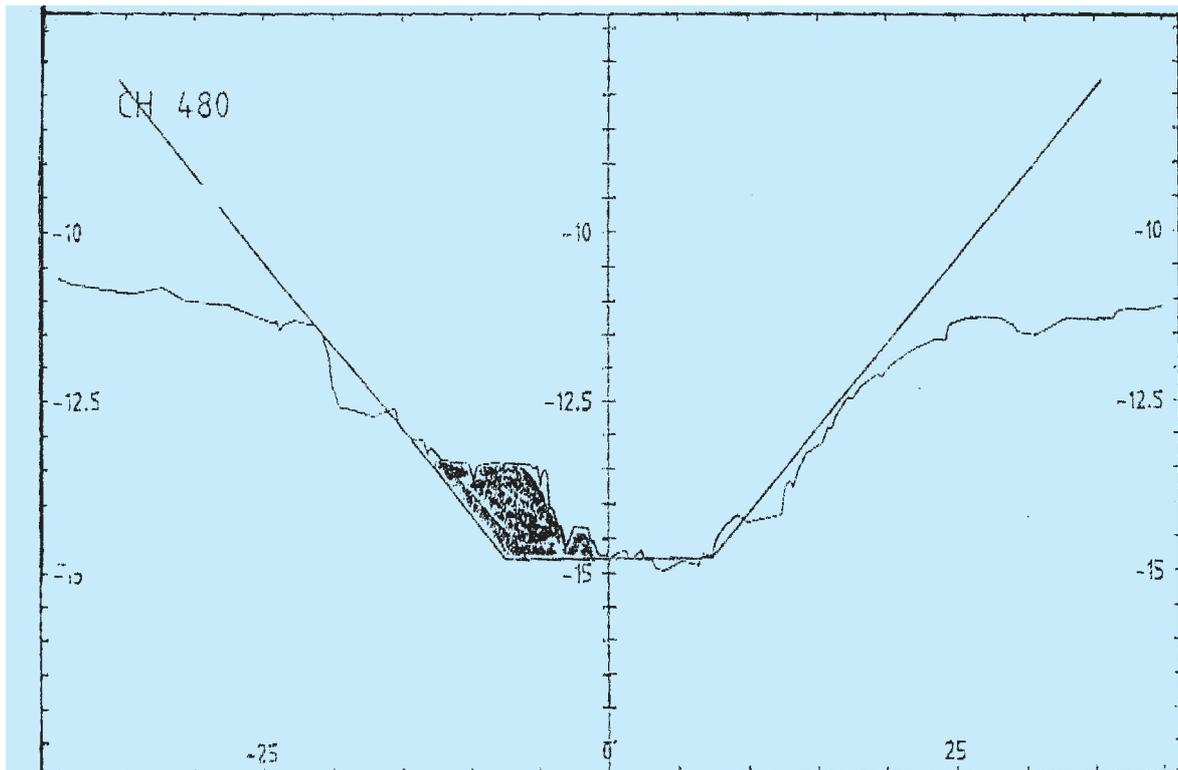
Figure 10. CH 480 cross-section. Preliminary outsurvey Kp 60-500, 15 November 1994, showing "hard spot".
