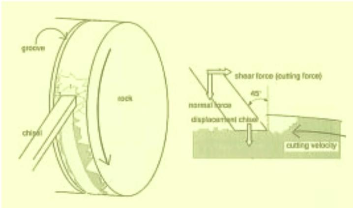
Figure 1. Scraping test.
