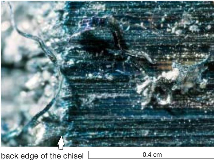
Figure 4. Part of a test chisel wear-flat worn in wear mode I.
