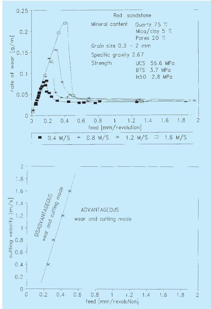
Figure 3. Rates of chisel wear in scraping tests on a sandstone as a function of the feed for different cutting velocities. At a higher cutting velocity a higher feed is needed for an advantageous mode of wear.
