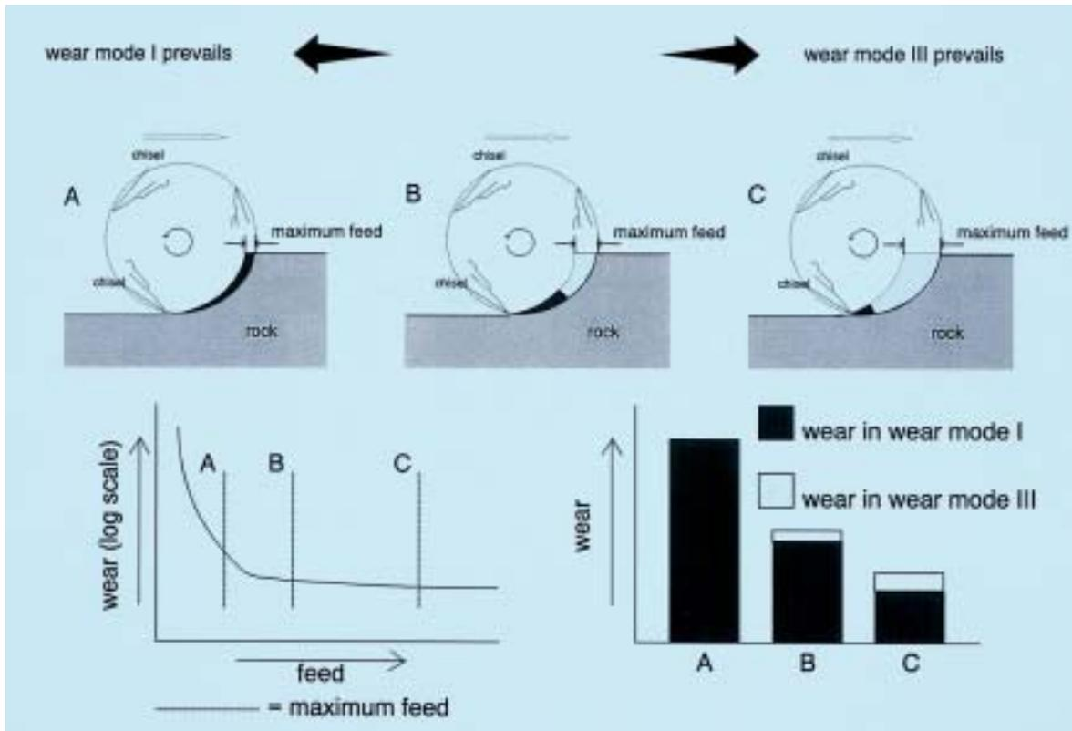
Figure 6. Wear at low feed (start of a cut) is higher than at higher feed (end of a cut). The wear during a cut is determined by the magnitude of the contribution of wear mode I.
