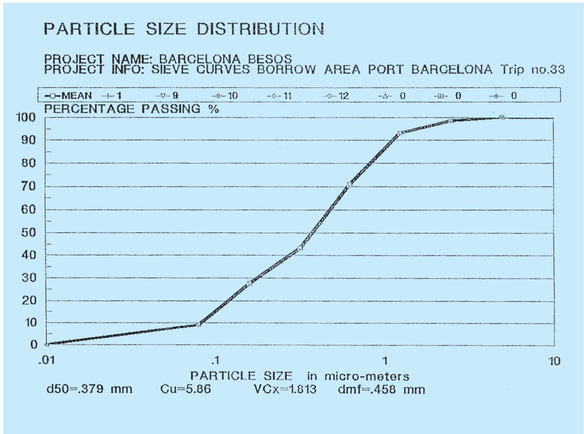
Figure 12. Particle size distribution of sand for backfilling.
