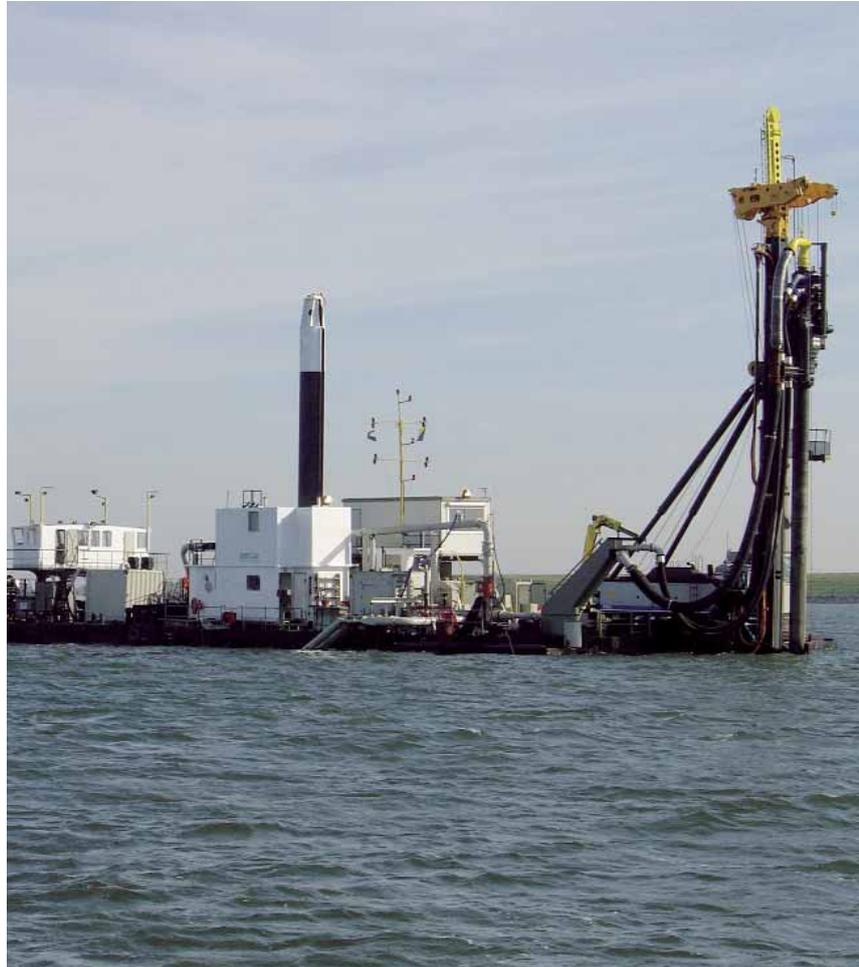
Figure 1. The BeauDredge® during construction of retention basin at the Herfterwetering.
