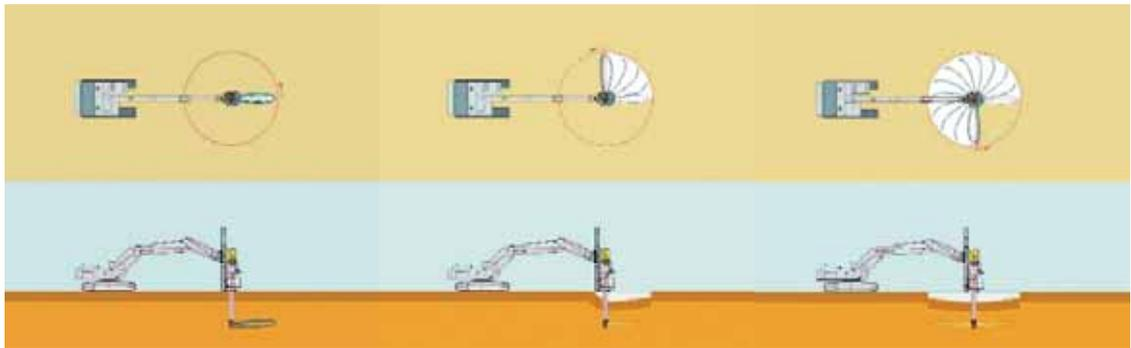
Figure 5. Steps 1 through 3 show the extraction of clean sand in circles from the layer underneath.
