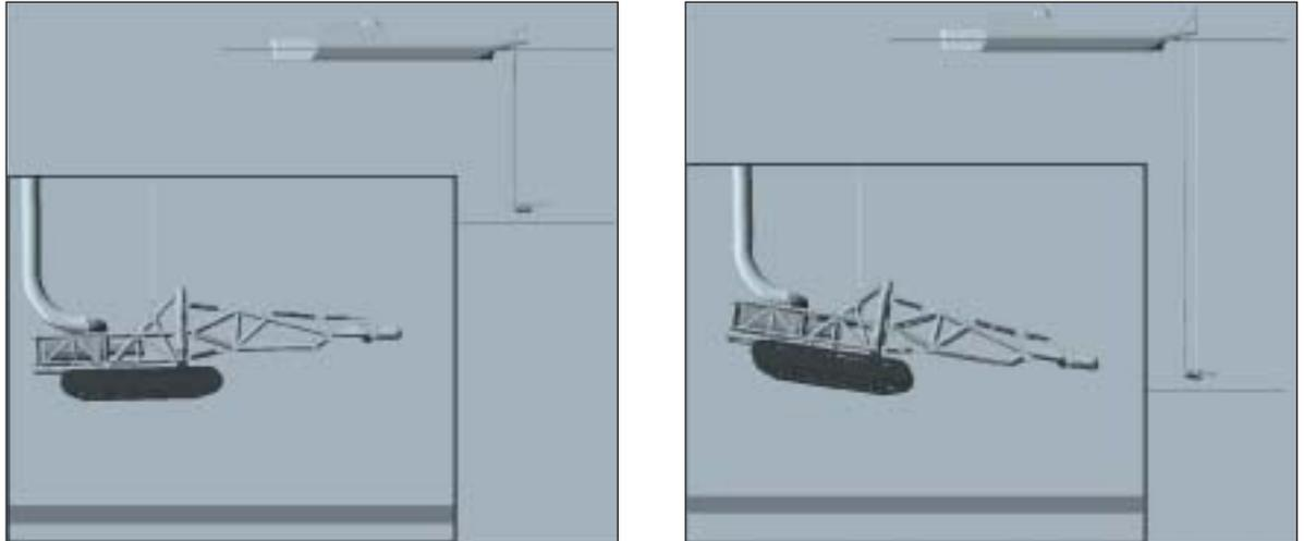
Figure 5. Static angle as a result of the buoyancy of the discharge hose (left 100 m, right 200 m) prior to modification of the hoisting point.
