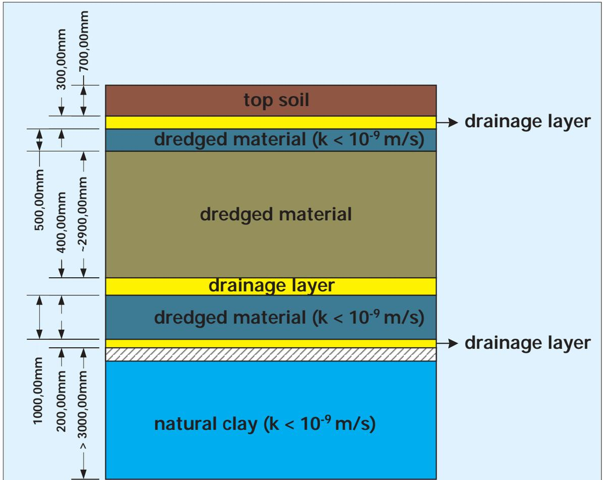
Figure 8. Structure of the dewatering fields and disposal site.
