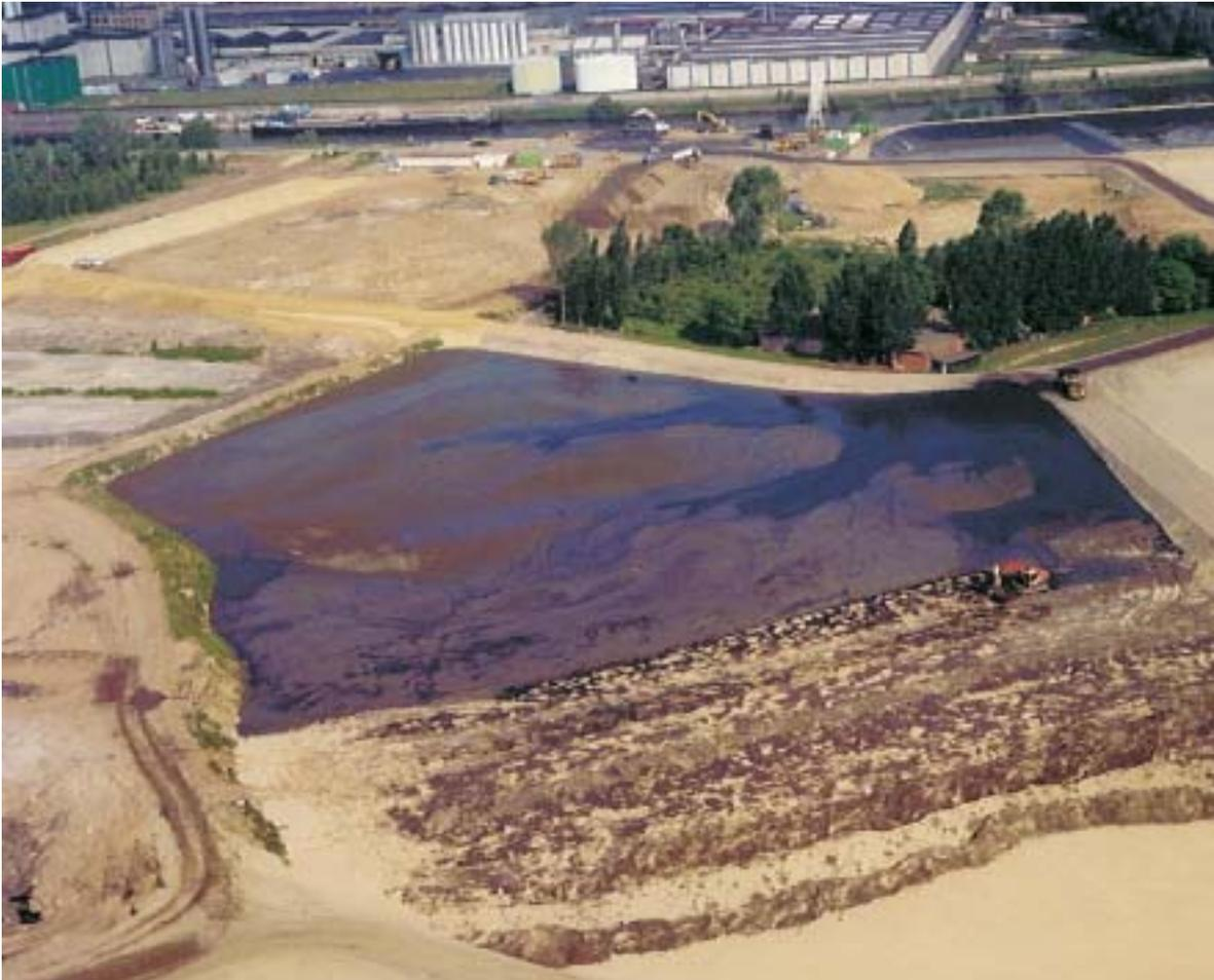
Figure 9. Accelerated natural dewatering of dredged material.
