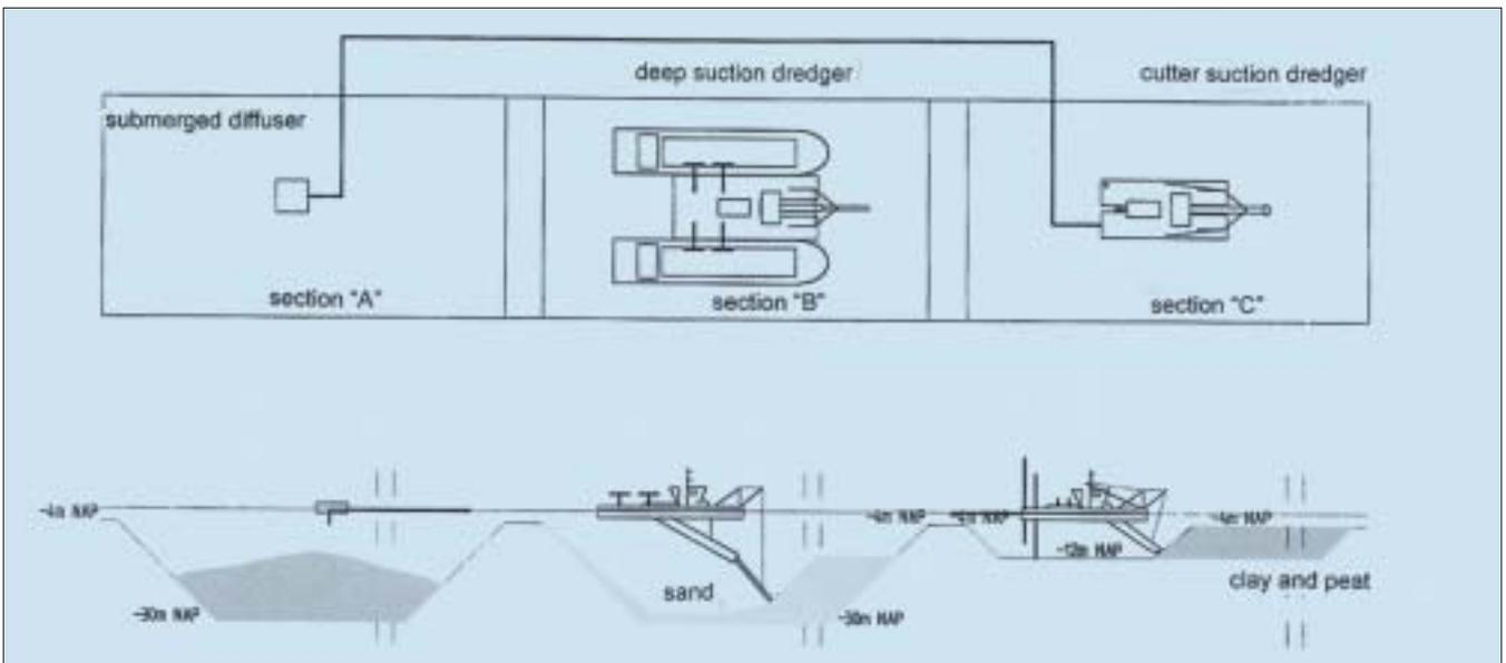
Figure 28. Diagram: top and side views showing the “train of dredging activities” in order to excavate the sand and relocate the overburden of clay. This method of dredging avoided the need for large temporary storage areas for the volumes of clay to be dredged. In the photograph (taken on 27 March 2002) the deep suction dredger Faunus and the cutter suction dredger Aegir can be distinguished.
