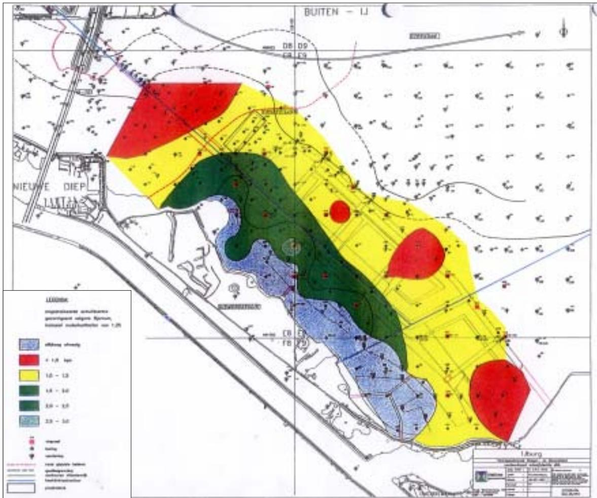
Figure 13. Contour map of the undrained shear strength (at depth 0.5 metre below bottom).
