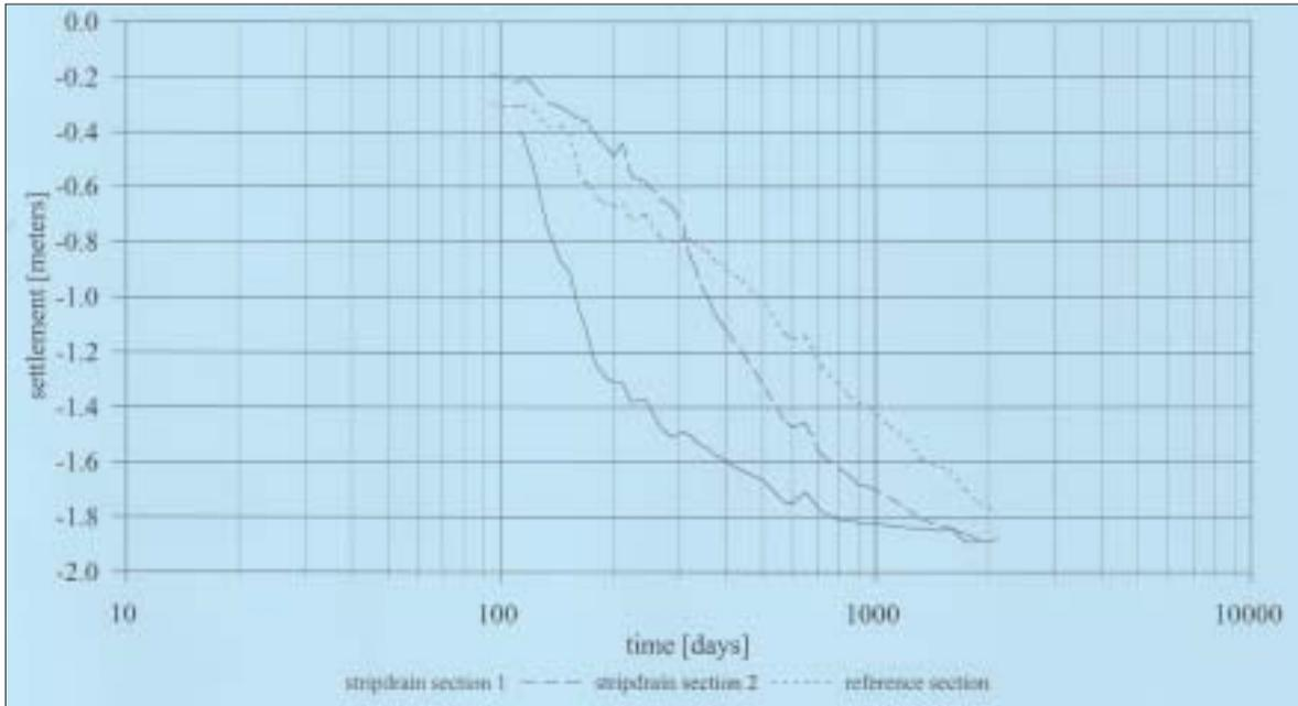
Figure 17. Pilot project: measured settlements versus time.
