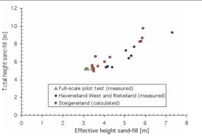
Figure 26. Effective versus total height sand fill.
