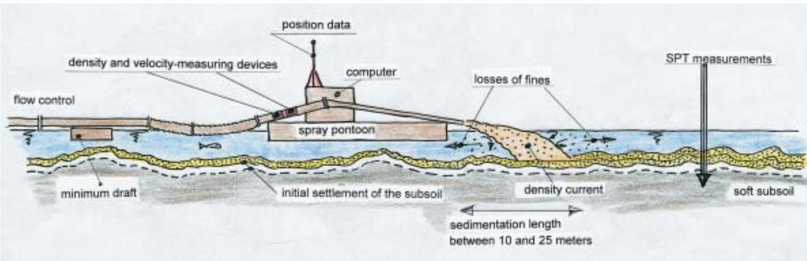
Figure 30. Schematic drawing of the spray pontoon "1208" and the process features of spraying sand as described in this article.
