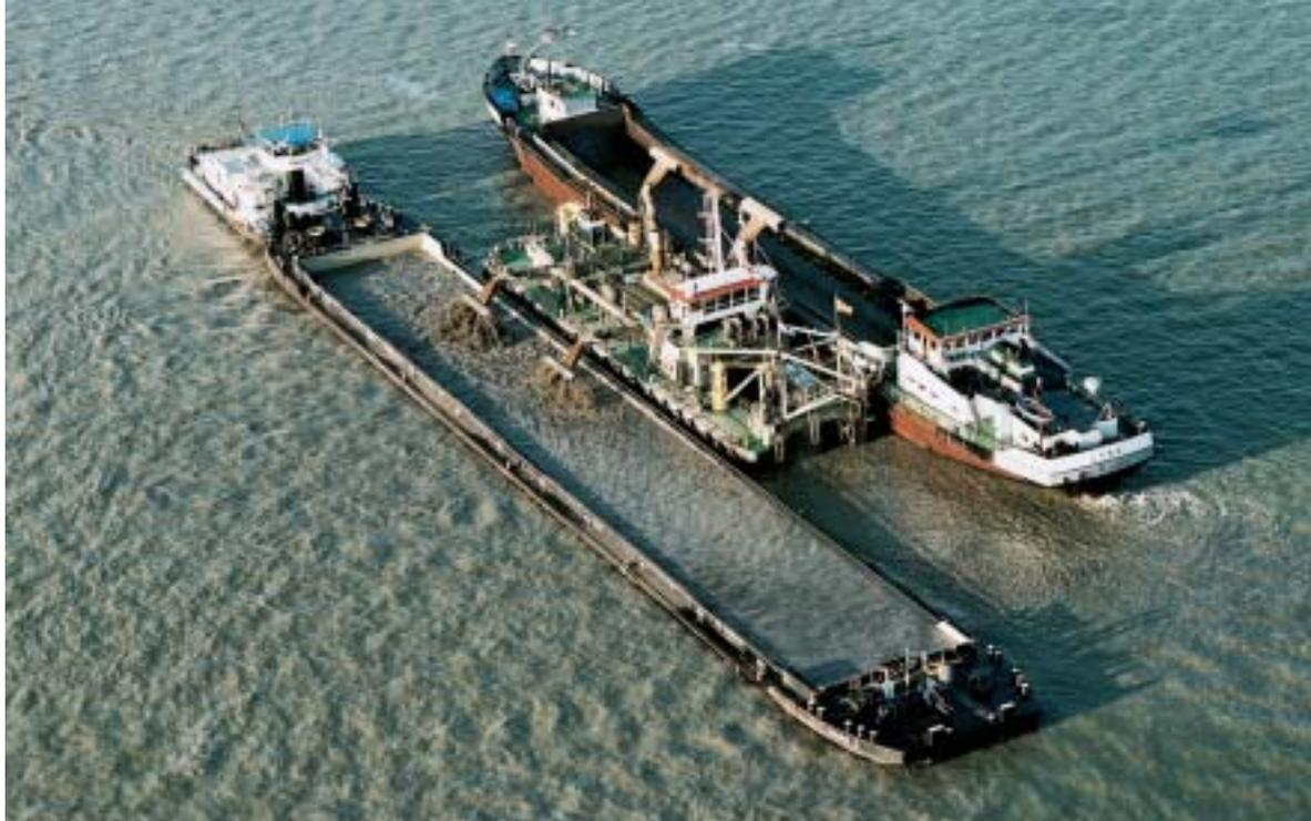
Figure 8. Deep suction and barge-loading dredger *Faunus* excavating up to 30-metre-deep sand at the borrow area (approximately 25 kilometres distance from the reclamation site) and at the same time loading transport barges of 2,000 cubic metres volume each. The sand dredging process was often disturbed as a result of the presence of clay lenses in the sand. Photograph was taken on 18 January 2002.
