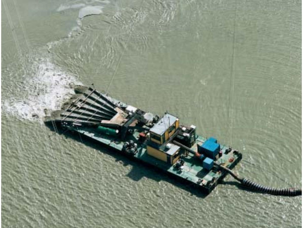
Figure 29. Computer-controlled spray pontoon "1208" for reclaiming sand in thin layers. The pontoon can work in very shallow waters. The sand-water mixture escapes the pontoon over a 12-metre-wide chute. The density and velocity of the mixture is measured on board. A computer calculates as well as controls the speed of the winches in order to reclaim with any desired constant layer thickness. Photograph taken on 29 April 1999.
