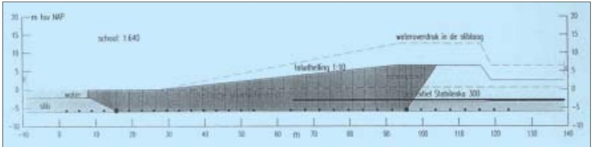
Figure 21. Steigereiland (Bastion): Results stability calculation Slope/w.
