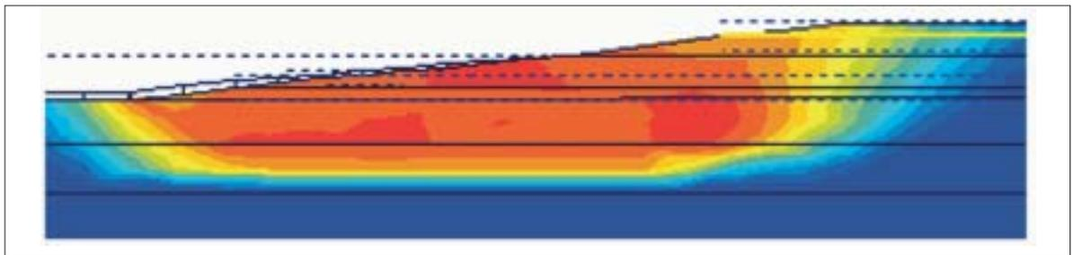
Until the installation of the vertical drains, the failure mechanism was mainly squeezing. The young Holocene clay layer squeezes over the firmer deeper layers. After consolidation and resulting strength improvement the failure mechanism transformed to a transition mechanism combining both circular and horizontal sliding. In Figure 21 and Figure 22 the results of the stability calculations from, respectively, Slope/w and PLAXIS are presented. The settlement and
