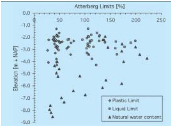
Figure 15. Left, Atterberg limits versus elevation.
