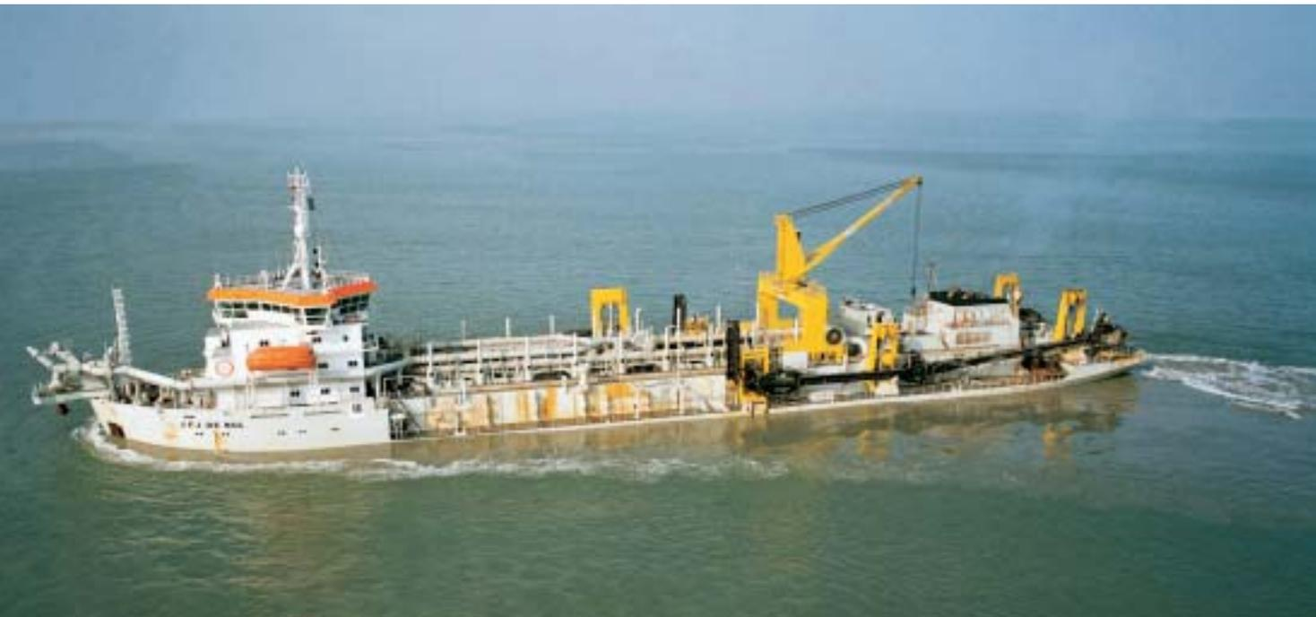
Figure 3. Trailing suction hopper dredger J.F.J. De Nul was one of two trailers used for pre-trenching operations.
