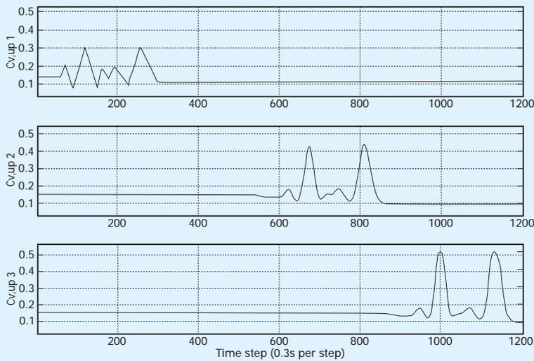
Figure 7. Deformation of density waves along the long pipeline (slurry velocity round the deposition limit velocity) observed at the inlet to the pipeline, 500 metres behind the inlet and 800 metres behind the inlet.
