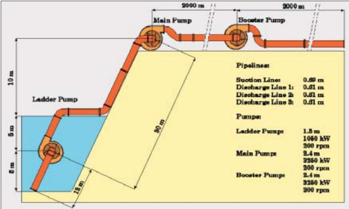
Figure 9A. The pump/pipeline system used.
