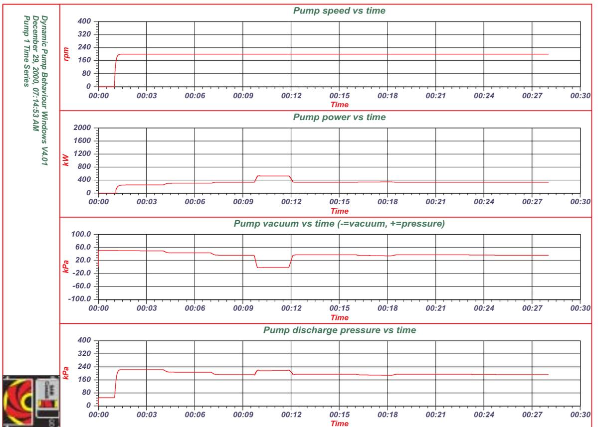
Figure 14. Speed, power, vacuum and discharge pressure of the ladder pump vs. time.
