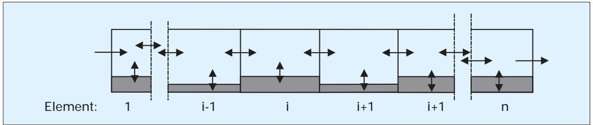
Figure 1. Elements of a pipeline filled with unsteady solids flow.
