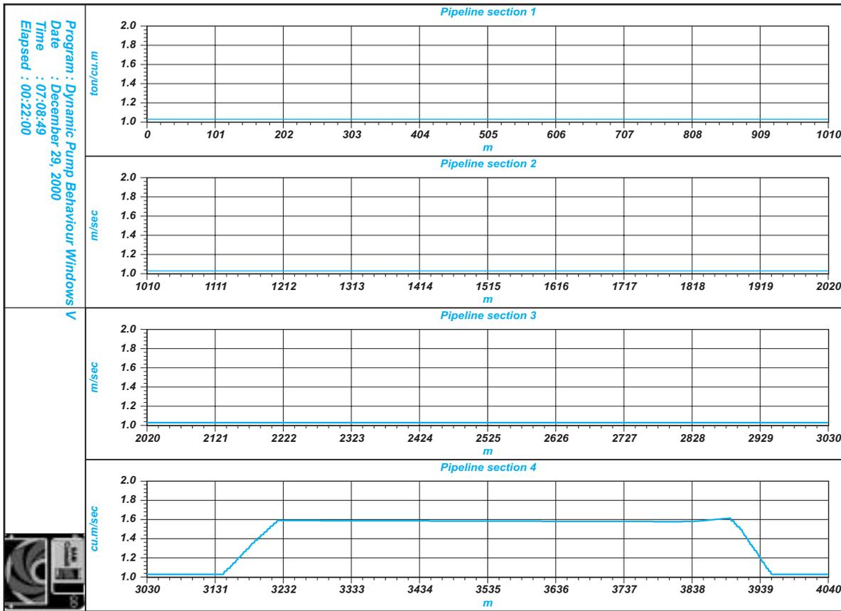
Figure 12. The density distribution in the pipeline after 22 minutes.
