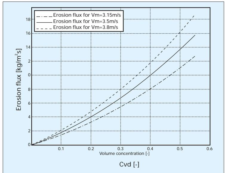
Figure 3. The erosion flux using the classical formula (Eqs. 4) for different solids concentrations and mean velocities of slurry in a pipeline.
