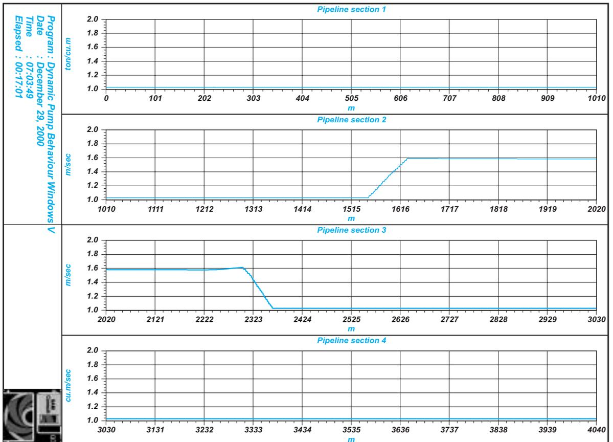
Figure 11. The density distribution in the pipeline after 17 minutes.
