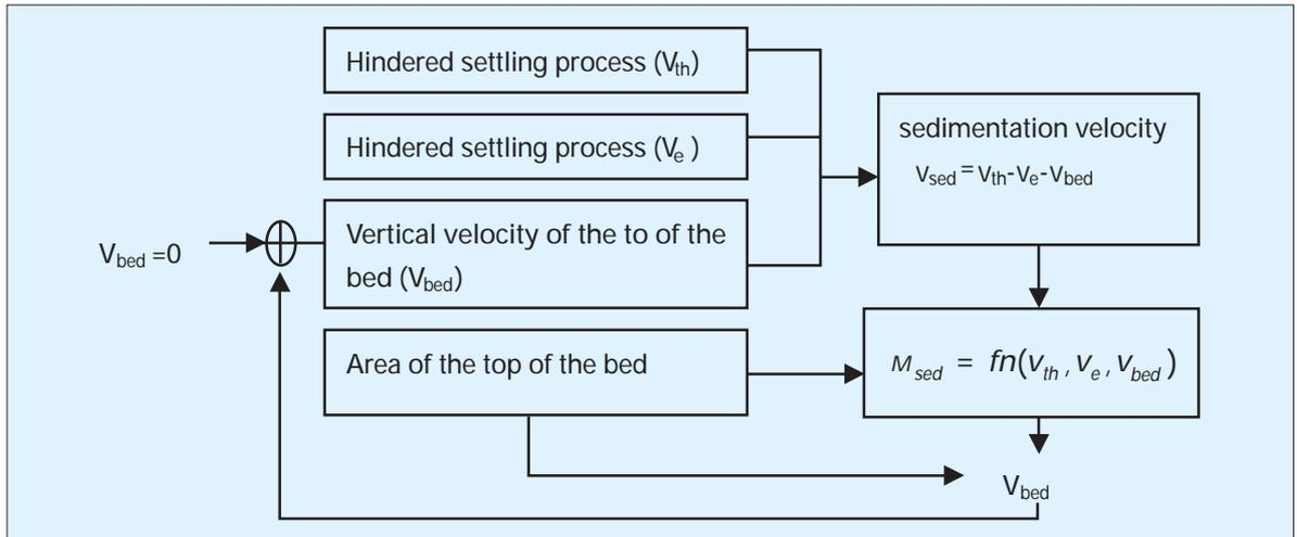
Figure 5. Computation of vertical mass exchange in the 2-D model.
