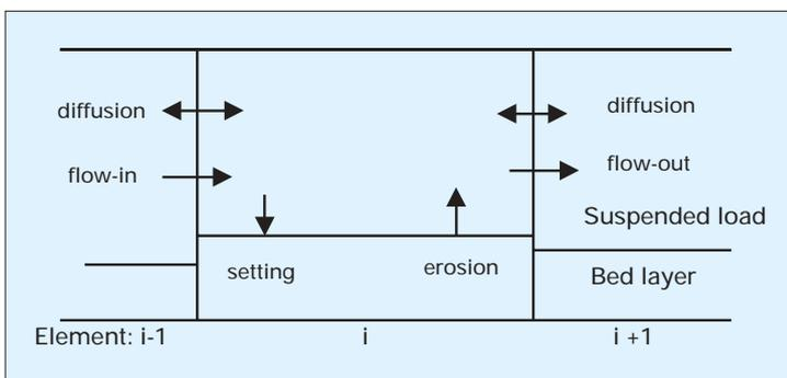
Figure 2. The transport phenomena simulated by the 2-D model.
