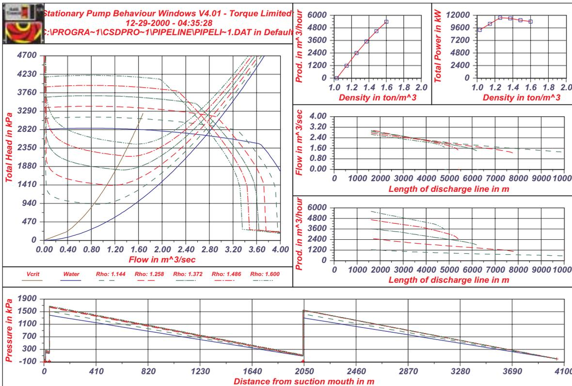
Figure 9B. Characteristics of the pump/pipeline system.
