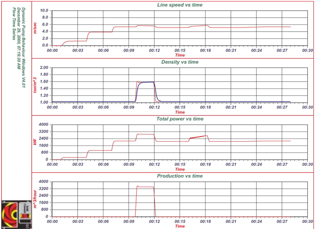
Figure 13. Line speed, density, total power and situ production as a function of time.
