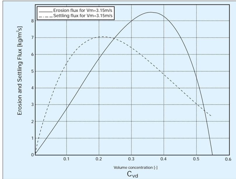
Figure 6. Comparison of settling and erosion fluxes according to the 2-D model in a 650-mm pipeline occupied by slurry of medium sand ( $d_{50}=0.25 \text{ mm}$ ) ( $V_m=3.15 \text{ m/s}$ ).
