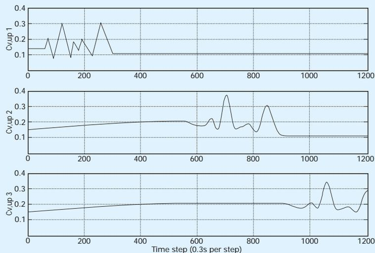
Figure 8. Deformation of density waves along the long pipeline (slurry velocity far above the deposition limit velocity) observed at the inlet to the pipeline, 500 metres behind the inlet and 800 metres behind the inlet.
