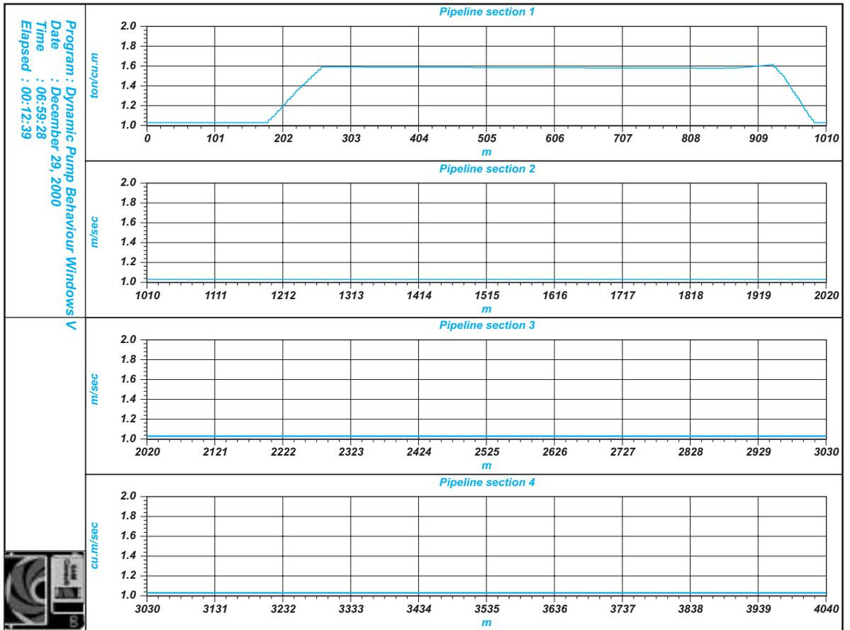
Figure 10. The density distribution in the pipeline after 12 minutes.
