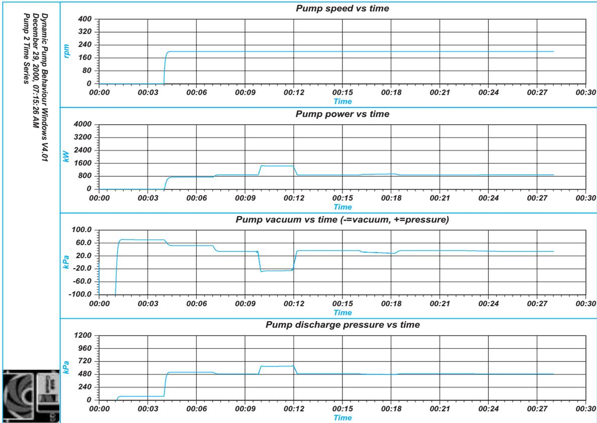
Figure 15. Speed, power, vacuum and discharge pressure of the main pump vs. time.
