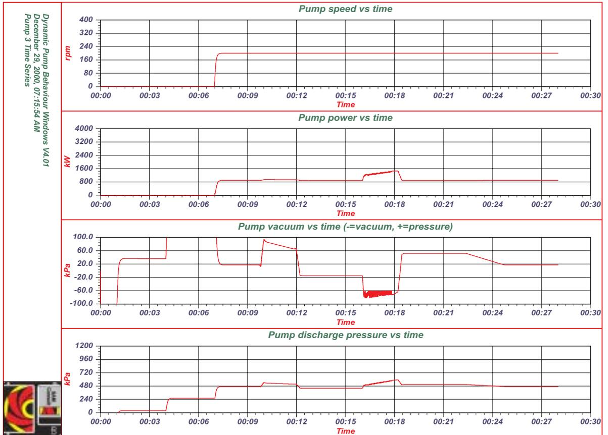
Figure 16. Speed, power, vacuum and discharge pressure of the booster pump vs. time.
