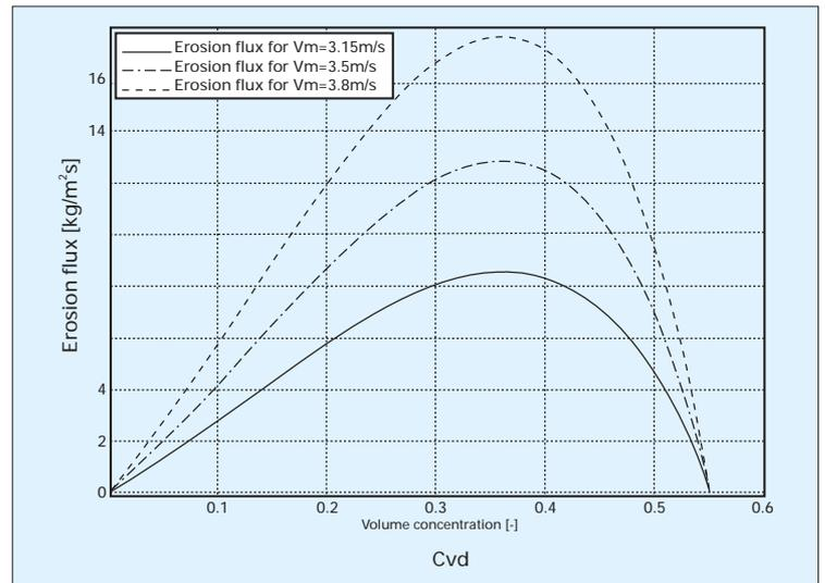
Figure 4. The erosion flux using the adapted formula (Eq. 7) for different solids concentrations and mean velocities of slurry in a pipeline.
