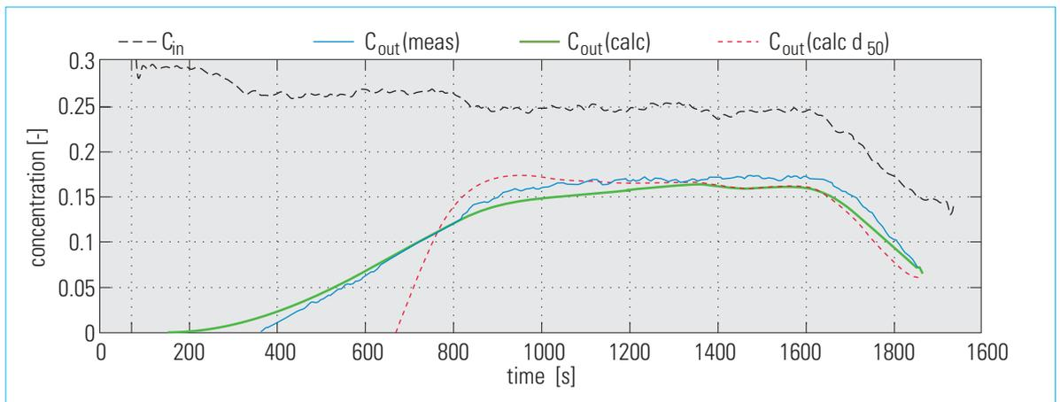
Figure 9. Comparison between measured and computed concentration during test 06.
