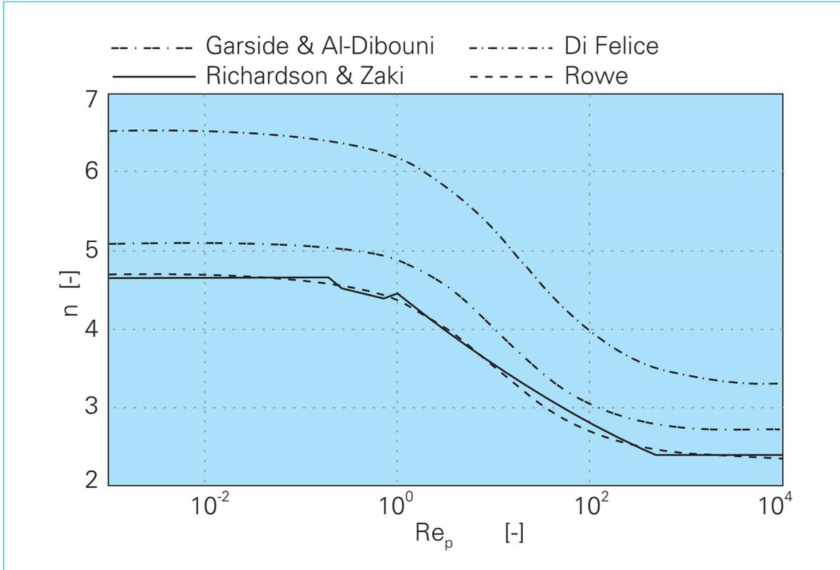
Figure 5. Exponent of hindered settling function.
