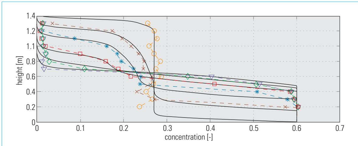
Figure 6. Calculated and measured concentration profiles at different times.
