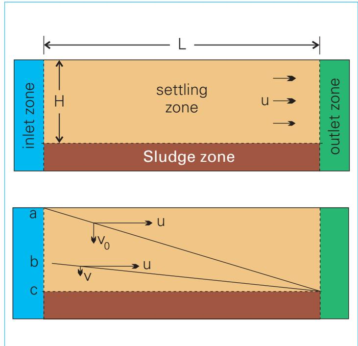
Figure 3. Simplified settling process according to Camp.
