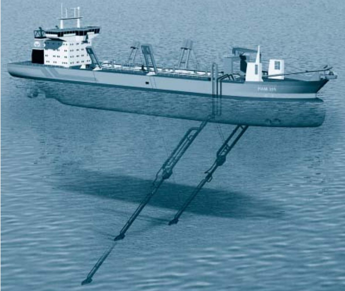
Figure 1. Artist's rendering of a trailing suction hopper dredger, with cutaway underwater showing suction pipes and hopper.
