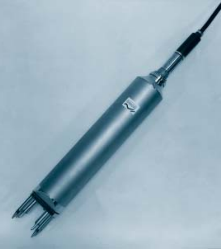
Figure 1. The NAUTISONDE probe. Mechanical data: Length, 68 cm; Diameter, 12 cm ; Mass, 23 kg (in air).
