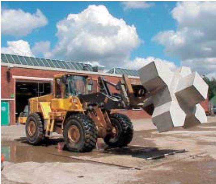
Figure 15. Stacking the Xbloc® for storage, after production and before placement.
