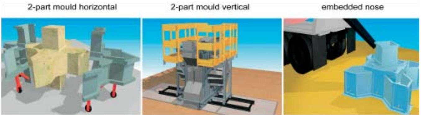
Figure 13. Various mould options for casting.
