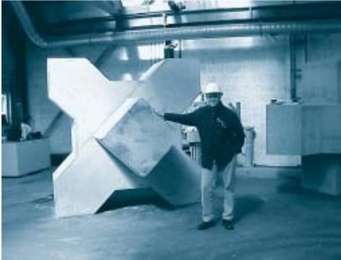
Figure 1. The 4 m<sup>3</sup> Xbloc<sup>®</sup> with one of the engineers.
