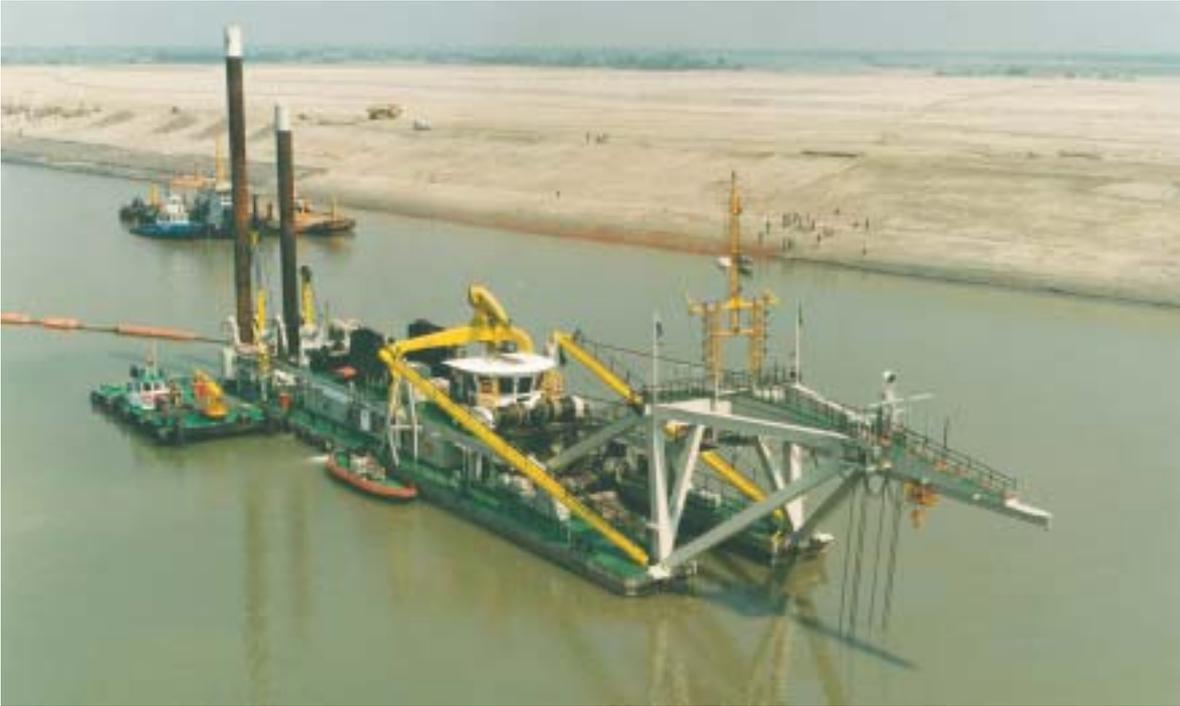
Figure 5. The bulk dredging for a new and deeper trench was performed by the cutter suction dredger *Jokra*.
