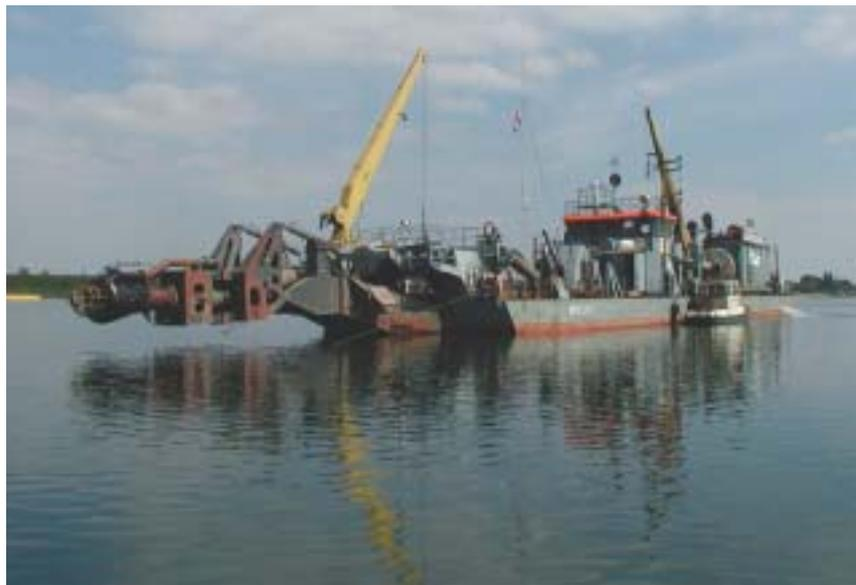
Figure 6. The suction dredger *Nordland* was mobilised by Boskalis' German subsidiary Heinrich Hirdes for the removal of siltation material from the trench.
