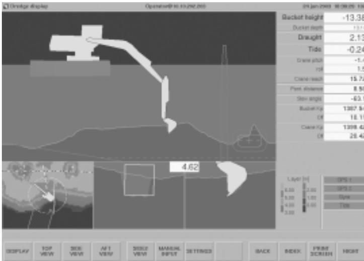
Figure 7. A view from the Rocky of the computer screens showing the crane monitoring system (CMS).
