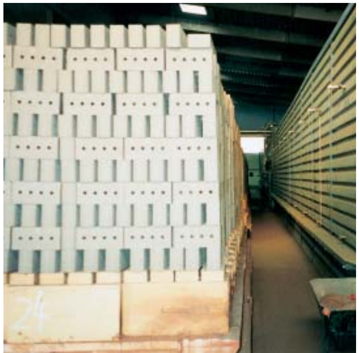
Figure 12. Synthetic bricks made from dredged materials, Hamburg, Germany.
