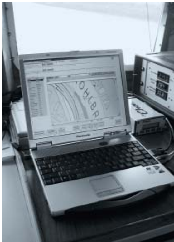
Figure 4. On-board computer for remote monitoring of the hopper dredger.
