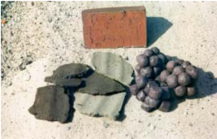
Figure 14. Products made from dredged material: sand, silt building material, bricks and blown clay-pellets
