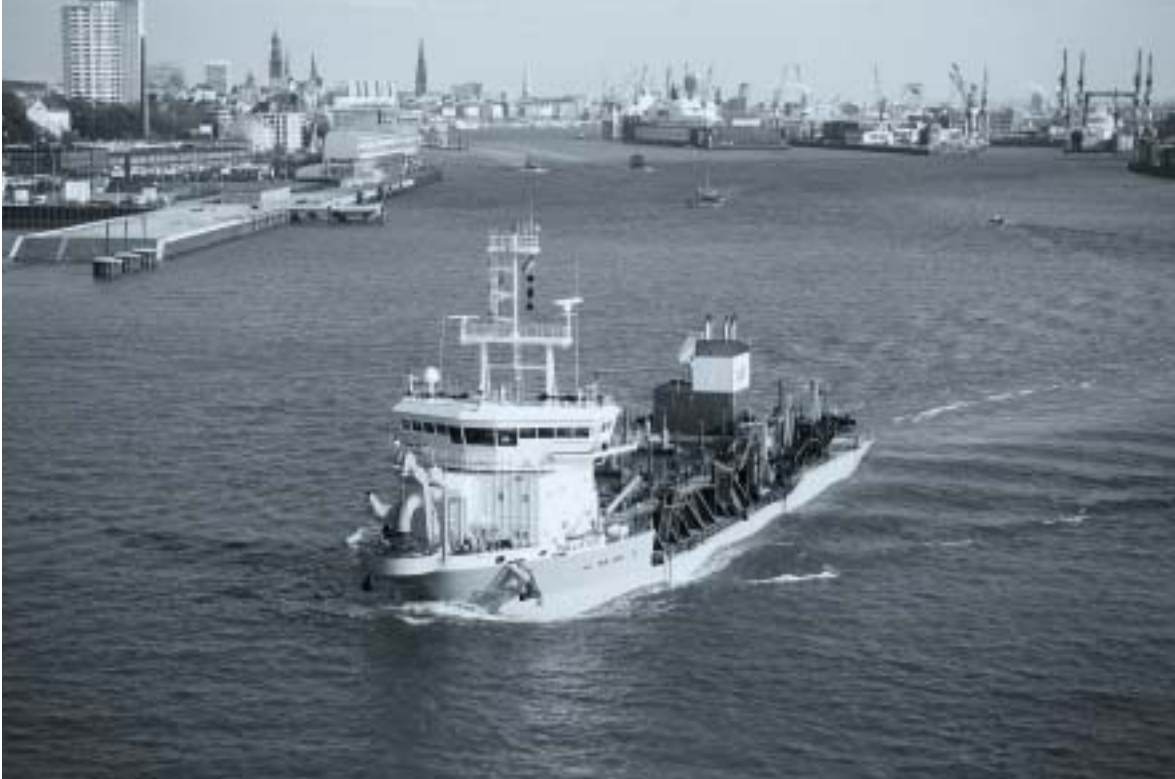
Figure 2. Hopper dredger in front of the port of Hamburg (source: Nordsee Nassbagger- und Tiefbau GmbH).
