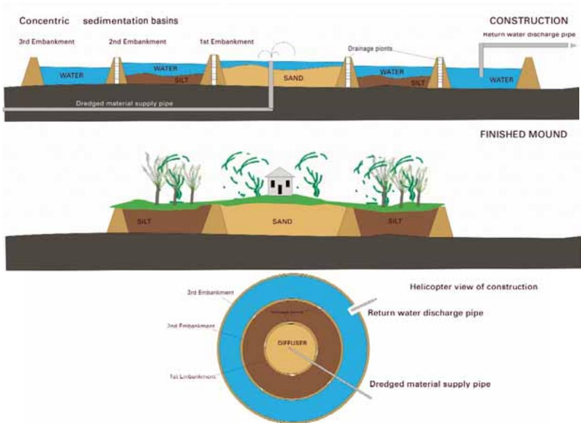
Figure 3. Concentric Sedimentation Basins (not in scale).
