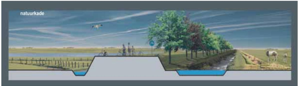
Figure 5. The “Watertight” design includes layered, compartmentalised embankments, partially made from dredged materials. These embankments allow better control of flood zones.
