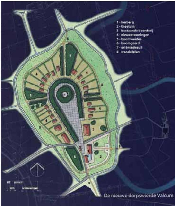
Figure 6. The “Werk met werk” idea creates a village on a mound, higher than the flood line, instead of living at a low level inside the protection of dyke walls.
