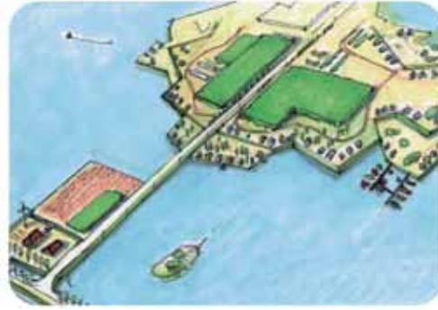
Figure 7. The two-stage idea of "Spaarkart" is (left) over 3 to 10 years widening an existing dike into a mound with earth-wall homes; and (right) a longer term (20 to 30 years) multifunctional mound where some 1,000,000 m<sup>3</sup> sludge are utilised.
