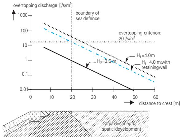
Figure 7. Overtopping discharge as function of the crest width, with and without retaining wall.
