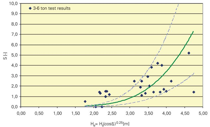
Figure 6. Comparison of 3D model test results with Theory of Galland.
