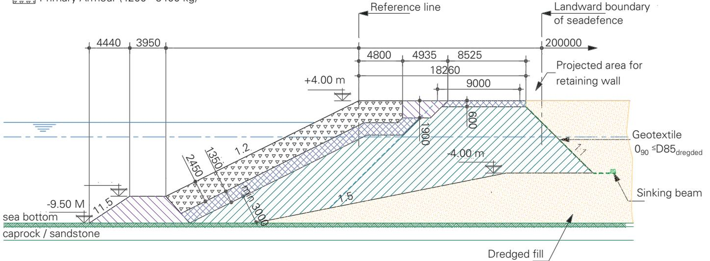
Figure 5. Typical cross section for Section I (4,750 m – 7,700 m).
