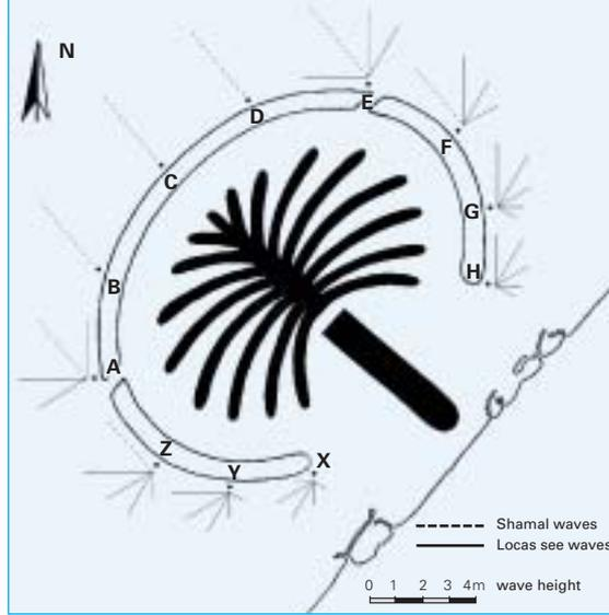
Figure 3. Wave heights at several points along the breakwater.
