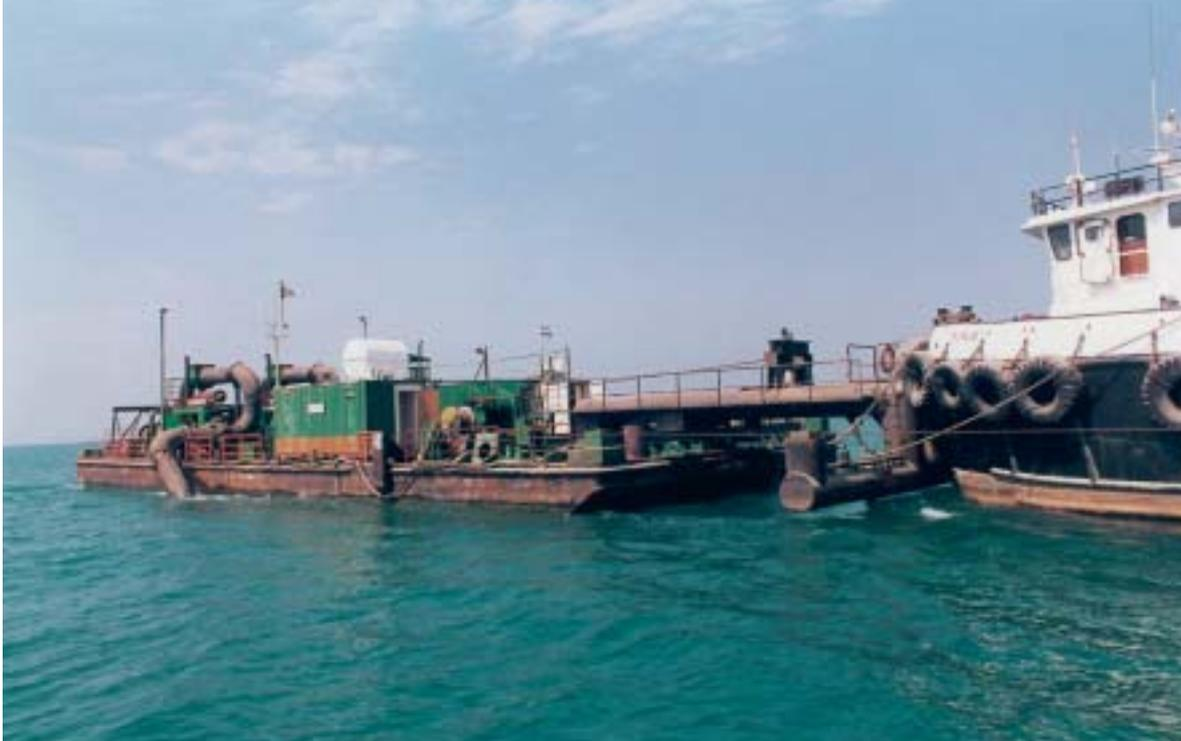
Figure 10. Water injection dredger Ham 924 at work.
