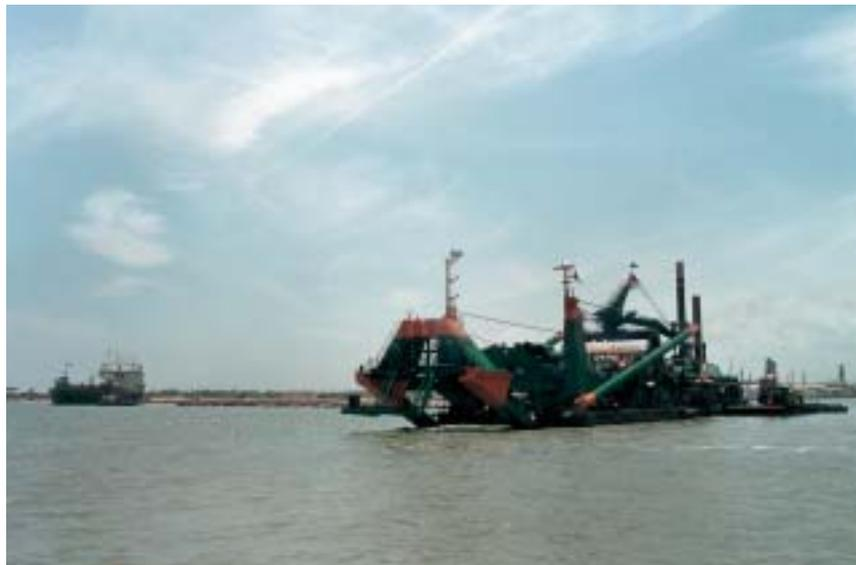
Figure 9. Double handling method in progress.
