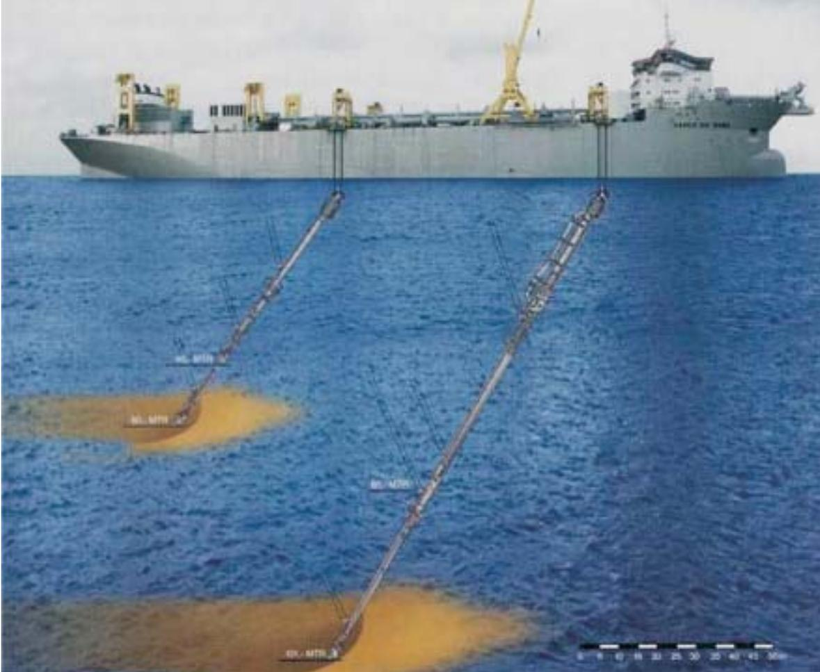
Figure 3. Schematic presentation of subtidal placement and water column recharge of fine-grained dredged material
