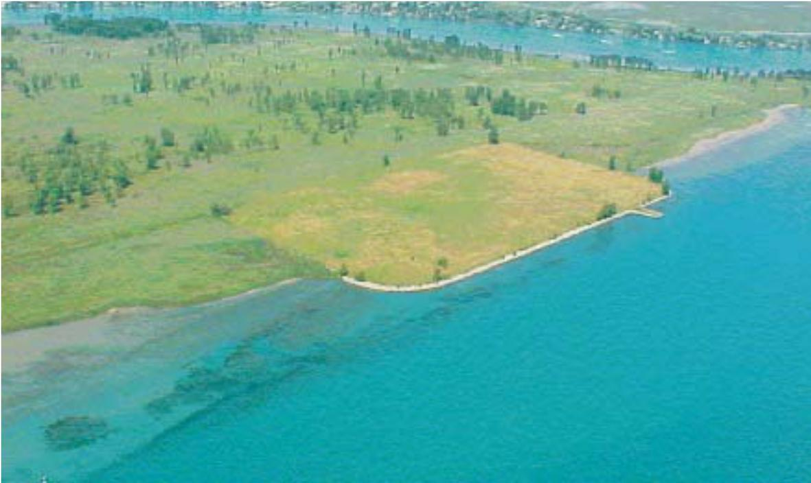
Figure 4. One of the long term engineered confined disposal facilities (CDF) on the adjacent Seaway Island for the disposal and management of material dredged from the SEB Cut-Off Channel.
