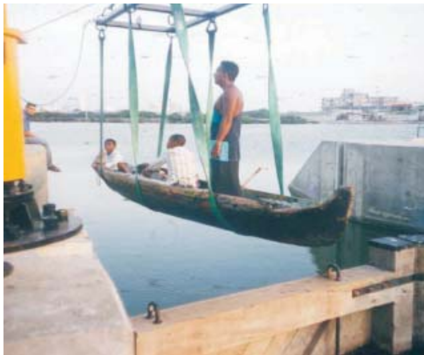
Figure 8. Small fishing boats are lifted by a derrick when the sluice is closed.
