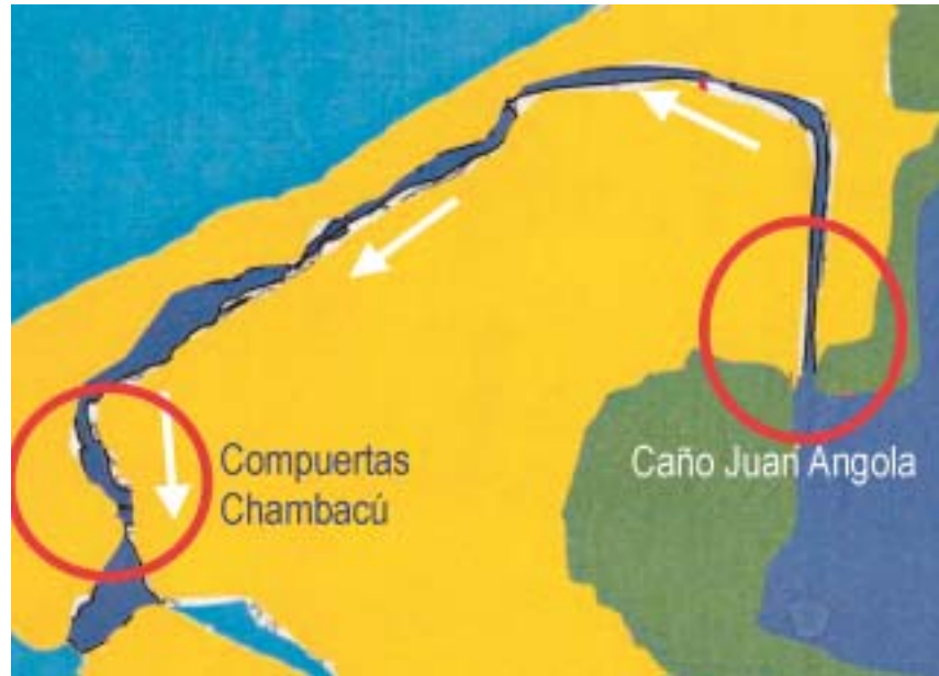
Figure 4. Map indicating the Caño Juan Angola and the one-way sluice at Chabacú which would allow only tidal outflow and prevent inflow.
