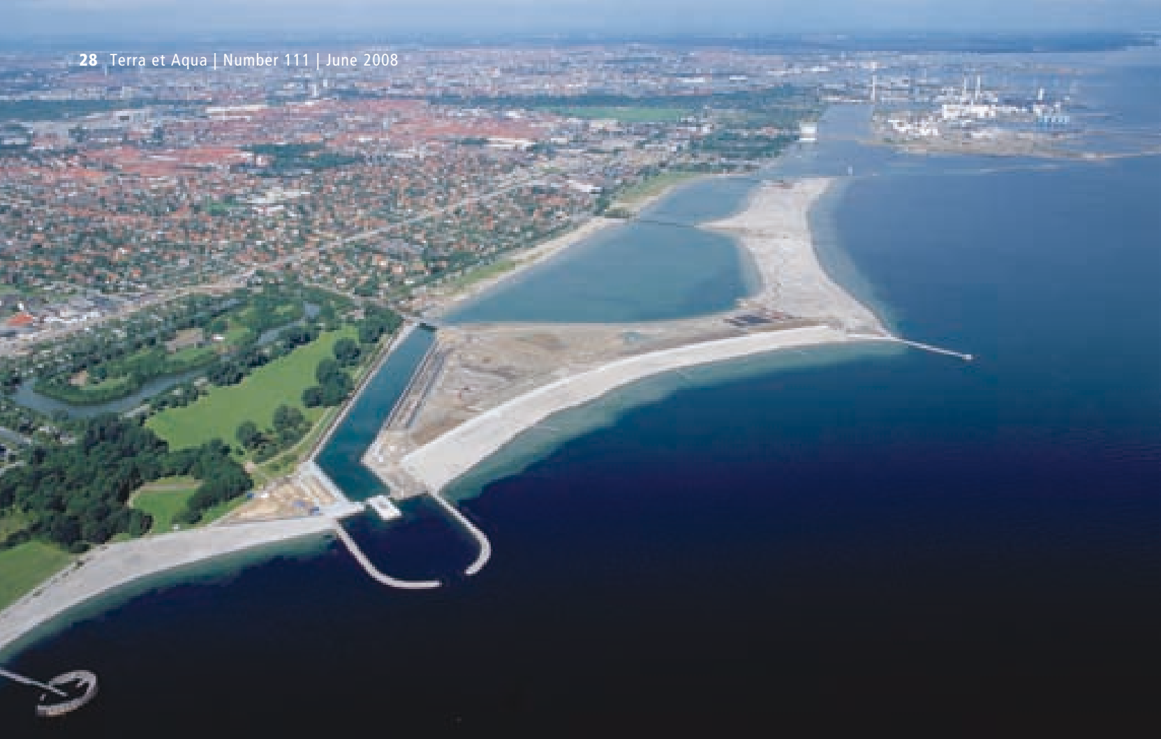
Figure 10. Aerial photo of Amager Beach Park, Copenhagen (courtesy of Jan Kofod Winther), which consists of the following main elements: Island with terminal structures north and south and a separating headland between northern and southern beaches and a lagoon. Designed by DHI, Hasløv and Kjærsgaard and NIRAS.
