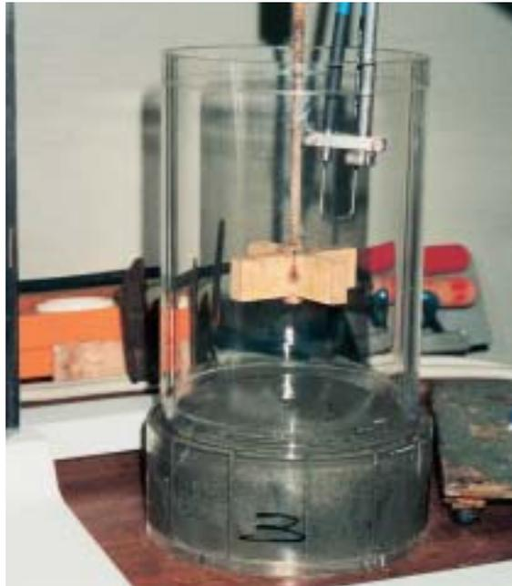
Figure 5. Prototype of the TACT (Turbidity Ability Criterion Test) device showing the agitation propeller, the silt sample underneath and the turbidity sensor above the propeller. With this test the sensitivity to resuspension of the water bed material can be derived in proportion to other water beds.
