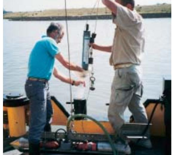
Figure 4. Taking site water samples of the background and turbid water with a NISKIN water sampler for laboratory analysis to enable the calibration of the turbidity sensors.
