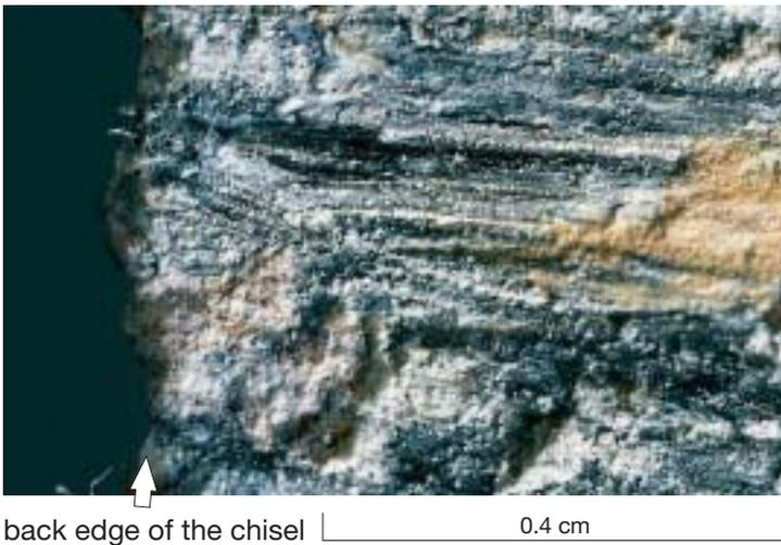
Figure 5. Part of a test chisel wear-flat worn in wear mode III.
