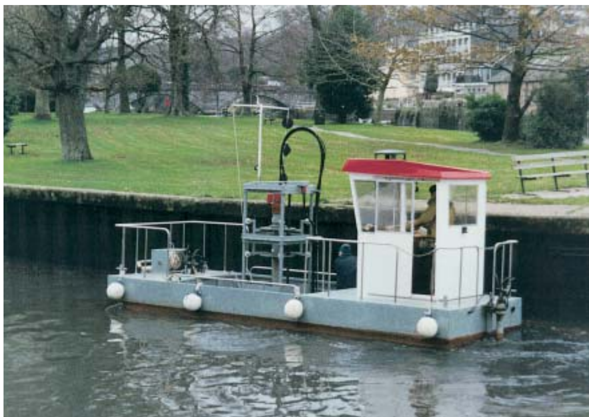
Figure 8. The agitation dredger Neptune alongside the quay, with its propeller down, agitating the sediments to allow silt to be dispersed by the tide.
