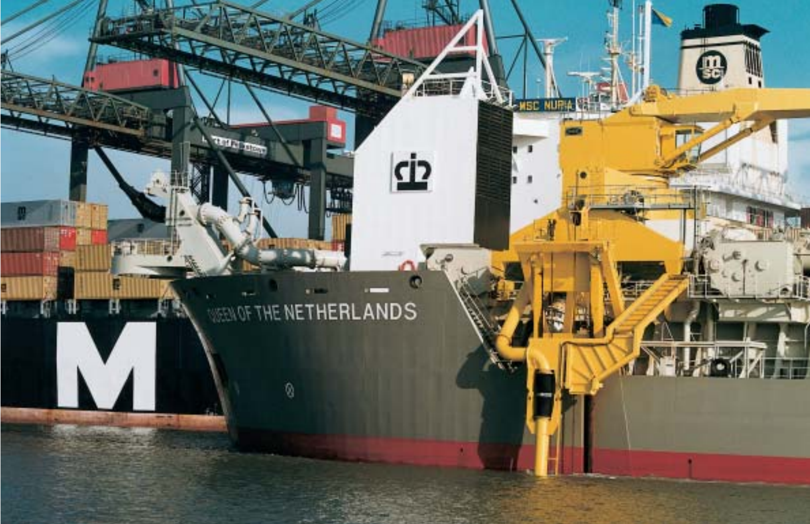
Figure 9. Trailing suction hopper dredger at work in the Harbour of Felixstowe, deepening the approach channel to make the harbour more accessible to the new generation of container ships.
