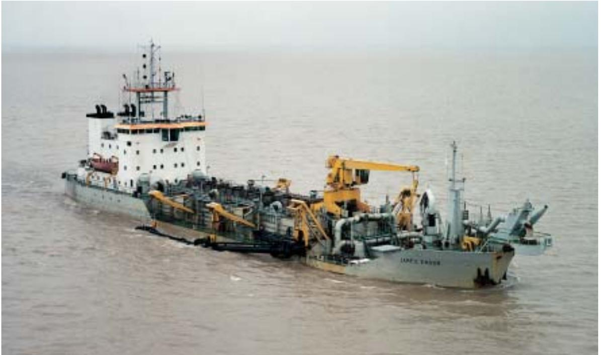
Figure 6. Several dredgers were used to dredge the River Plate, including (above) the trailing suction hopper dredger James Ensor.
