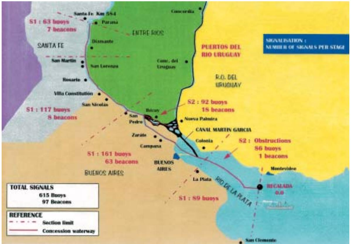
Figure 3. Signalisation system was adapted to international standards. This drawing of the River Plate indicates the number of signals (buoys and beacons) per stage (S1, S2).
