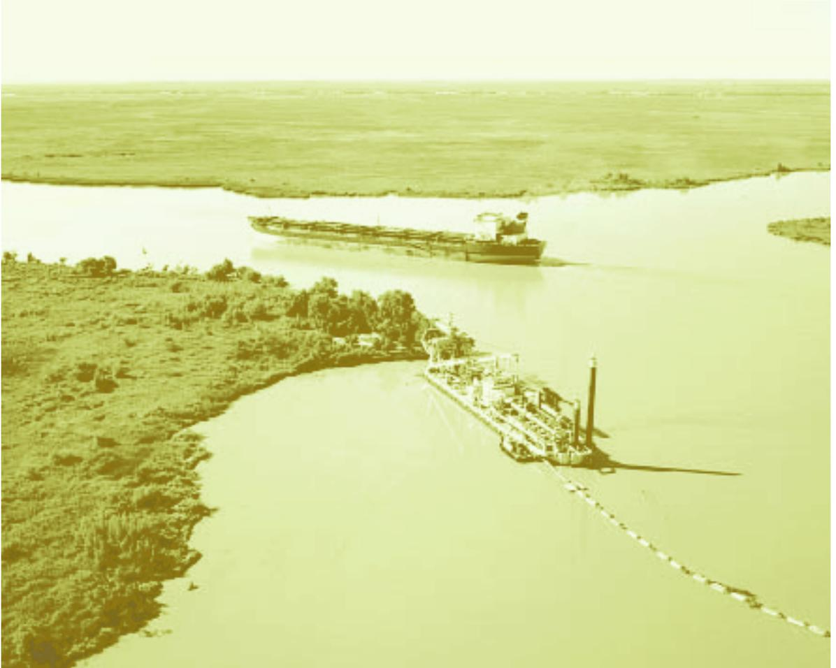
Figure 1. Maintenance dredging on the River Plate in the foreground; shipping traffic in the background.
