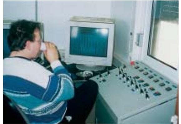
Figure 11. The unmanned dredge is controlled by one operator from the shore station using standard personal computers for visualising and controlling all the processes and PLCs for the signal input and output.
