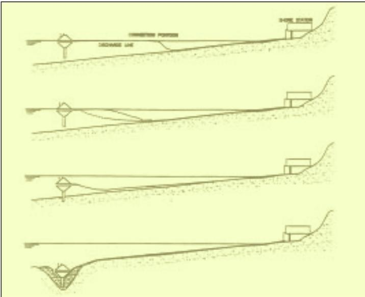
Figure 3. Drawing of the Punaise dredging process.
