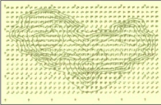
Figure 12. Depth contours of dredge pit at maximum area. Dredging was limited to -25.00 m MWL, and the resulting pit was kidney shaped.
