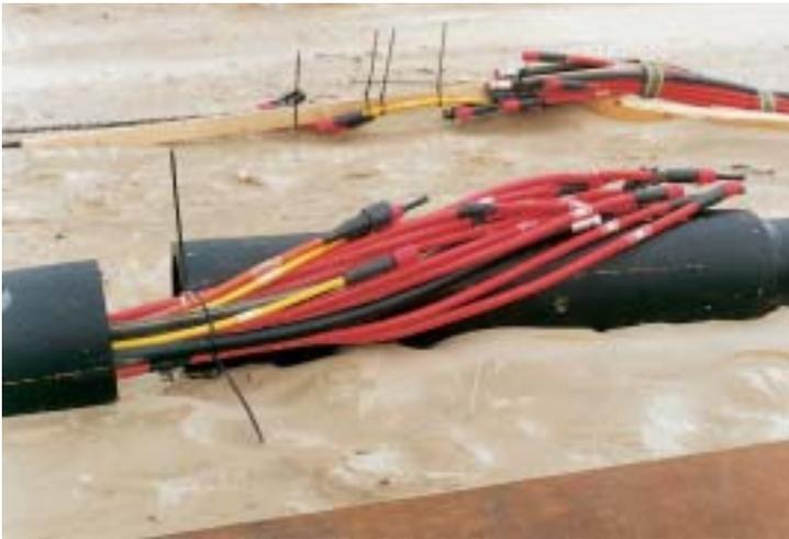
Figure 10. The umbilical contains 11 mm core diameter electrical cables, a relatively cheap and flexible system.
