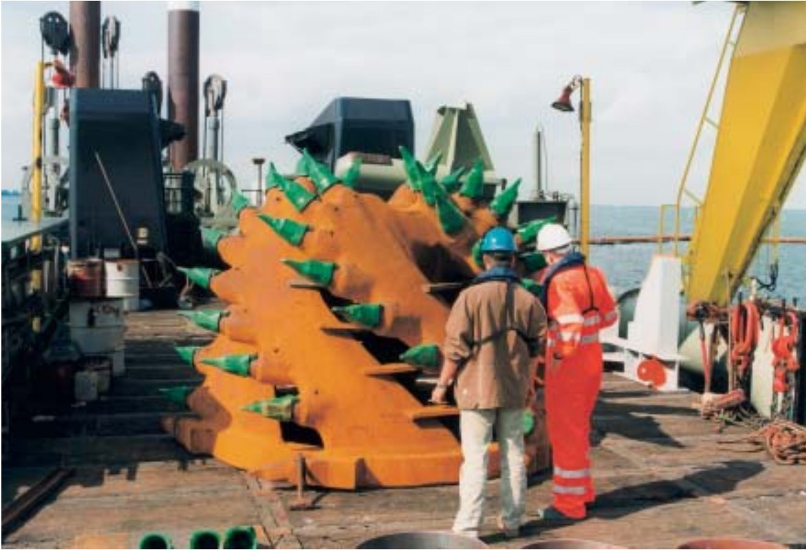
Figure 6. One of six cutterheads available at the project prior to being installed to dredge the extremely hard layers of Copenhagen Limestone in the tunnel trench.
