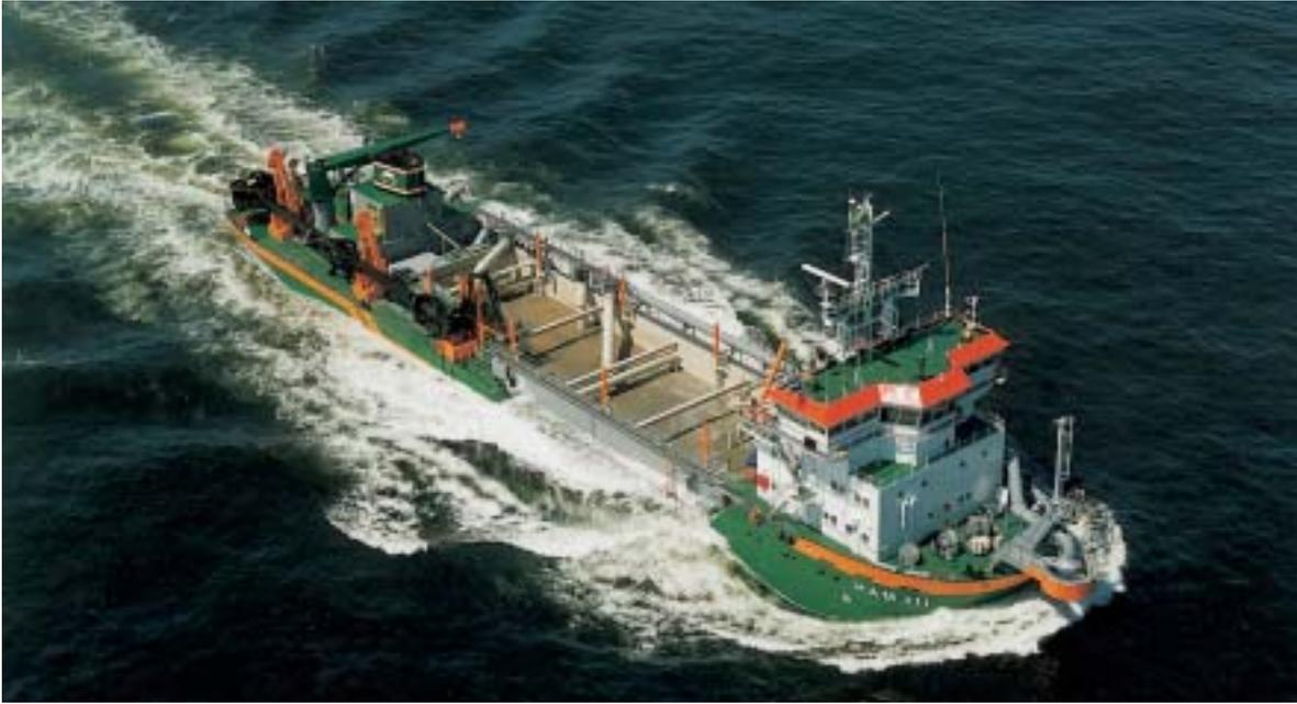
Figure 5. The HAM 311, a shallow draught trailing suction hopper dredger, is dredging the downstream area.
