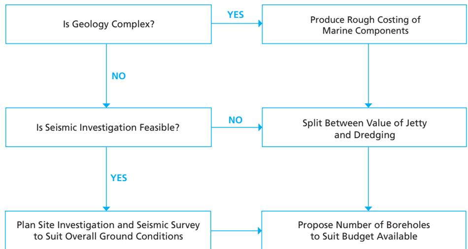
Figure 8. Proposed system to define the number of boreholes to characterise dredged areas relative to other marine components.
