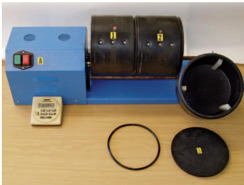
Figure 5. Laboratory tumbling equipment is sometimes used to simulate the degrading of sediment during dredging.
