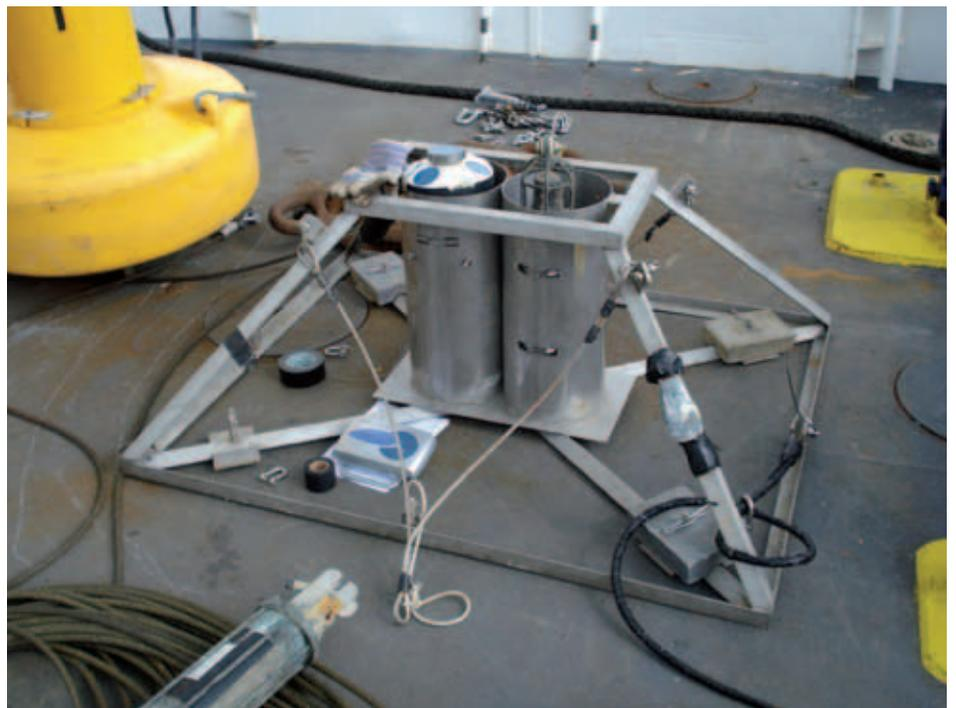
Figure 2. An acoustic instrument (Nortek AWAC, used for the measurement of currents and waves in the marine environment, is one of many tools for gathering essential geotechnical information.
