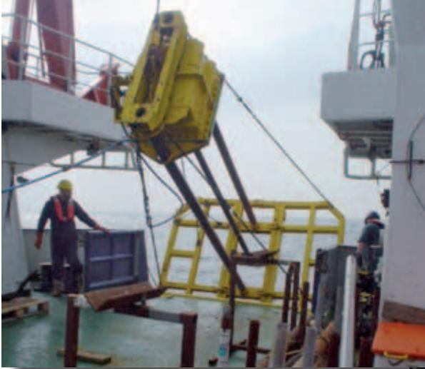
Figure 3. A Vibrocorer in use during site investigation works.
