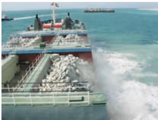
Figure 5. *Ham 602* in action as a stone-dumping vessel.
