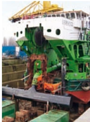
Figure 9. On the bucket dredger *Adriatico*, a T-shaped pipe was placed on the lower part of the ladder covering almost the total width of the pontoon.
