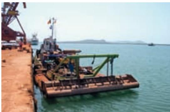
Figure 7. The Tug *Geer* working as a bed leveller.
