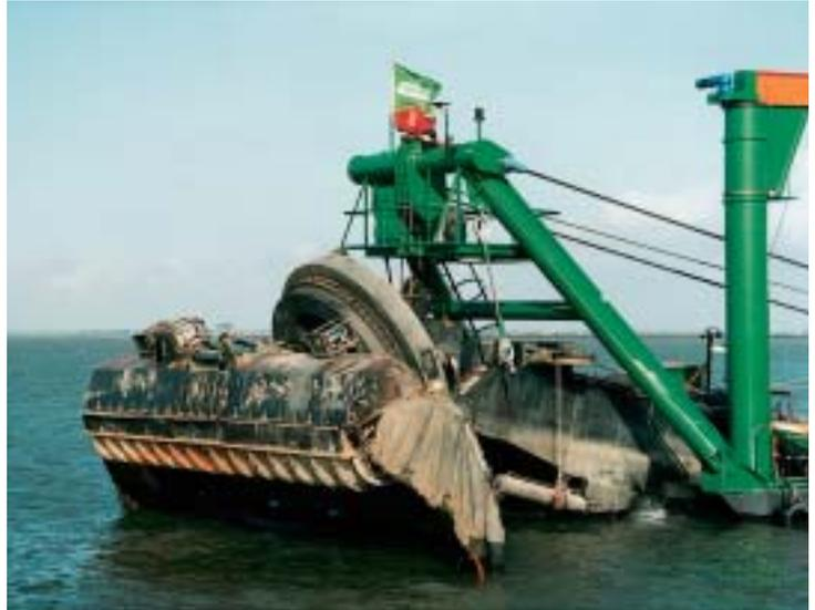
Figure 14. The auger and attached turbidity screen of the HAM 291, one of the dredgers which was specially developed for this type of sanitation dredging.
