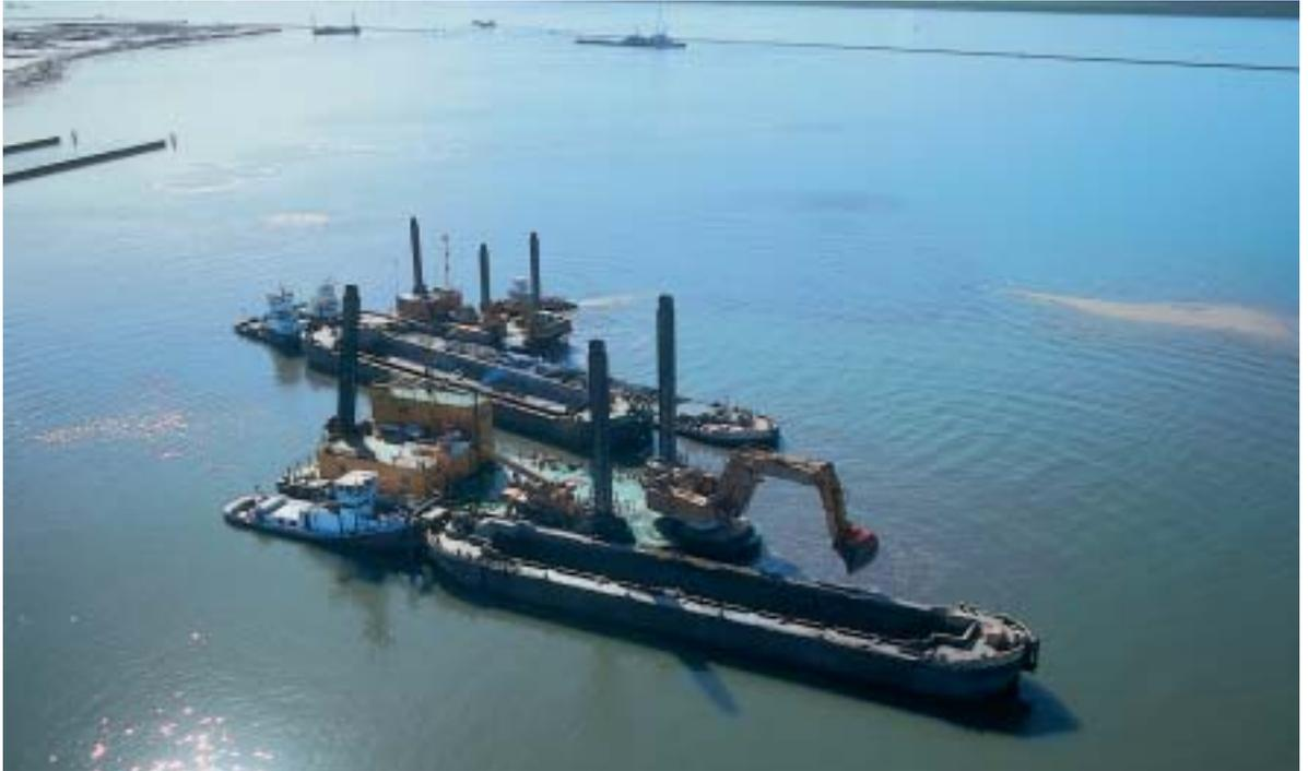
Figure 15. Backhoe dredgers *Manu Pekka* and *Kuokka Pekka* excavating Holocene material. With their buckets of 13 and 8 m<sup>3</sup>, and sophisticated bucket position indication system, they were very suitable for high production excavation (Rob de Wind bv).
