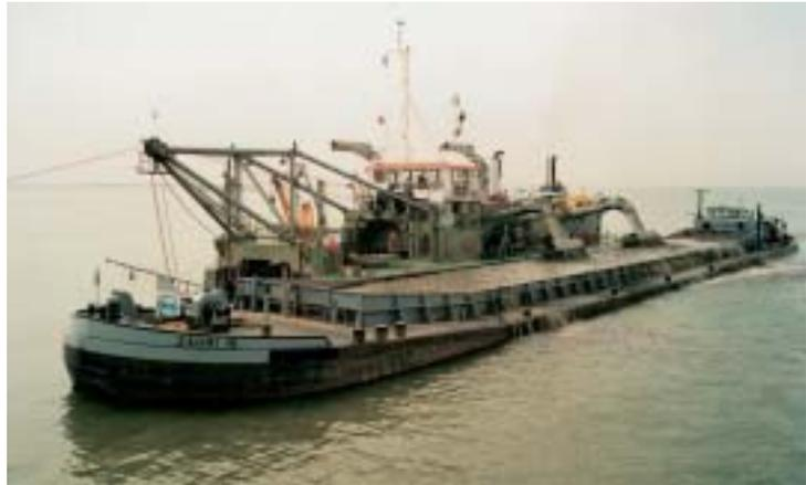
Figure 18. The suction dredger Faunus loading a self-propelled barge. Built in 1972, the Faunus has a remarkable track record in deep suction dredging in the IJsselmeer area, producing up to 2500 m³/hr.
