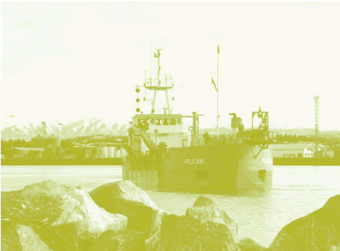
Figure 2. The *Pelican* is a split-hopper trailing dredger, equipped with a suction installation allowing the dredged spoil to be discharged ashore. The dredge pump has been mounted halfway along the suction pipe enabling the vessel to dredge highly concentrated mixtures at great depths.
