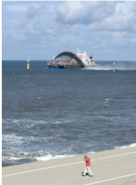
Figure 2. Twenty million cubic metres of sand were placed on the Dutch coastline to strengthen the Hondsbossche and Pettemer Sea Defences in north-western Holland. The sailing distance to and from the extraction site must also be considered in evaluating the CO<sub>2</sub> footprint.
