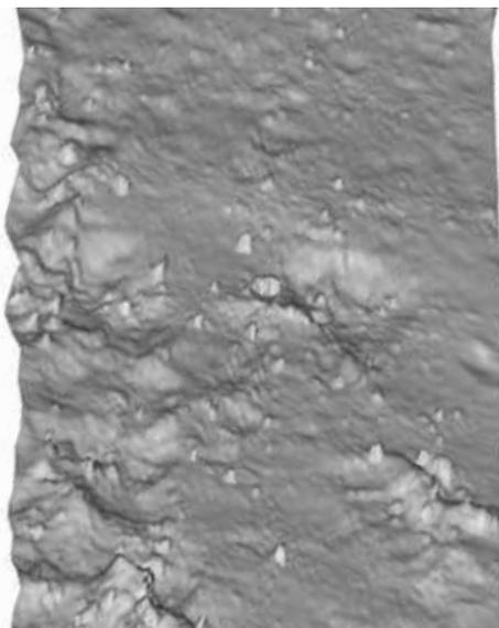
Figure 12. Survey results for rocky bottom: This is a sample of data from a project with a rocky bottom. Note that multiple passes do not create the "sounds" or "plowed field" look shown in Figure 11.
