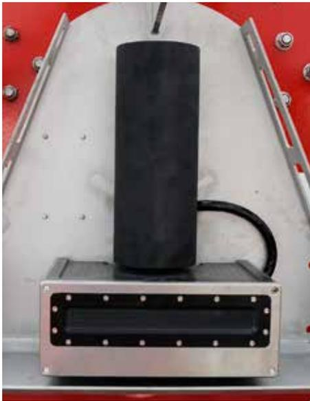
Figure 2. A modern multibeam sounding system.
