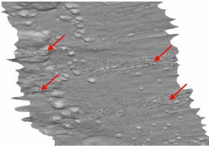
Figure 7. Survey area footprint showing effect of quartering waves.
