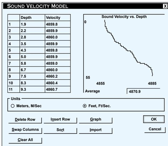
Figure 3. Screen shot of a sound velocity profile showing the variations in sound on the water surface and at the bottom.
