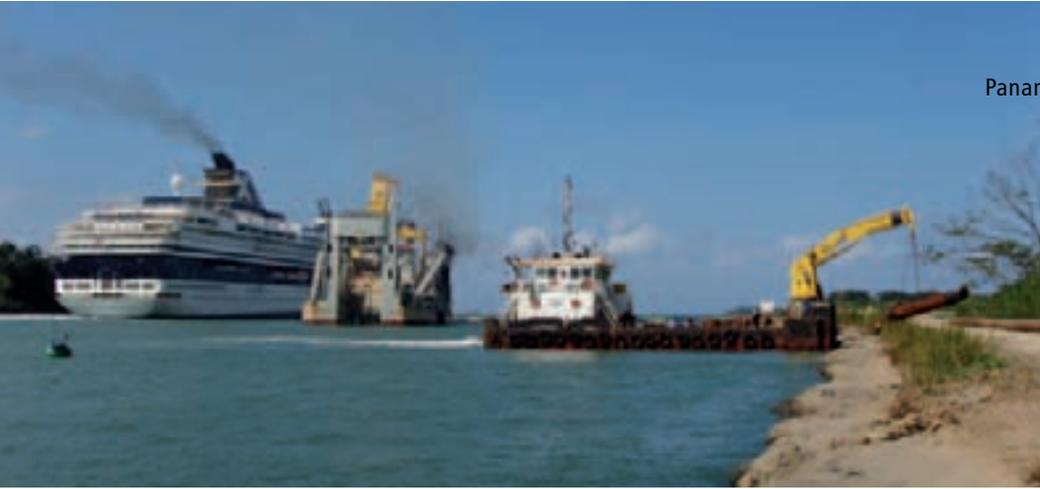
Figure 5. CSD *JFJ De Nul* working at Atlantic Entrance simultaneously with transiting vessels.
